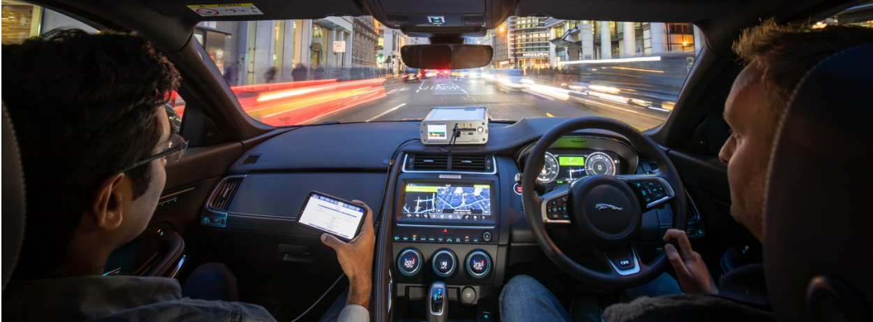
Figure 4. A Keysight GSS6450 is used to record the signal environment in a deep urban location
