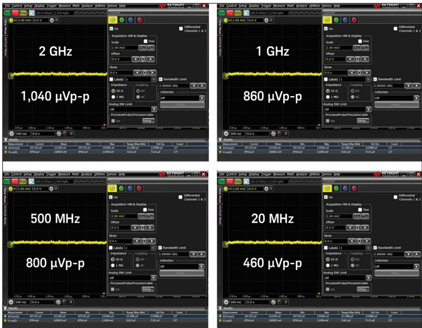
Figure 7: Baseline noise at various bandwidth limits with the Keysight N7020A power rail probe and MXR-Series oscilloscope.
