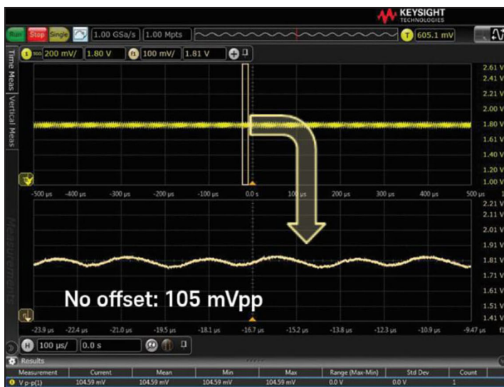
Figure 9: Measuring the noise on a 1.5 V DC supply with no offset and with the use of probe offset.
