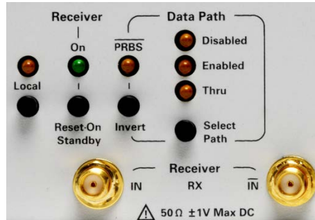
Figure 10. N4962A front panel – local, receiver, and data path controls
