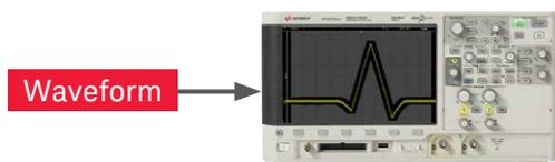
Create a mask with arbitrary margin around the reference waveform.
