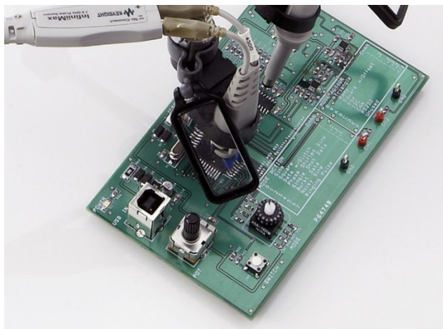
Figure 3. See a close-up view of the probing contact through the included 3X magnifying glass
