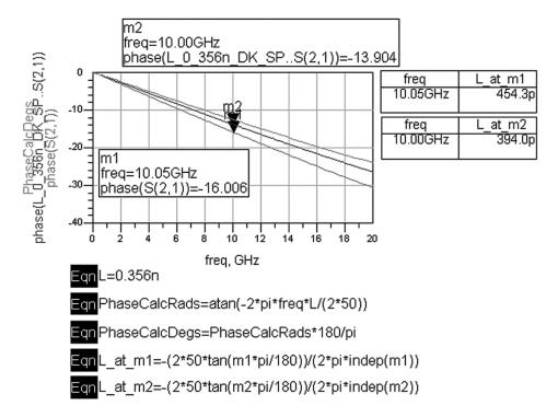
Figure 43. Comparing the phase shift of an ideal, DemoKit (equation-based), and Momentum-simulated inductors.
