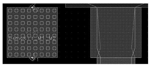
Figure 45. Original Metal1-to-Metal2 via structure at left, and after simplification for more efficient meshing, at right.
