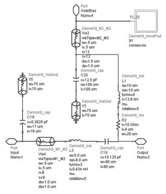
Figure 15. Input matching circuit schematic, with design kit elements and a DC bias network.
