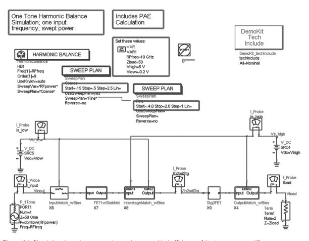
Figure 24. Simulating the gain compression and power-added efficiency of the two-stage amplifier
