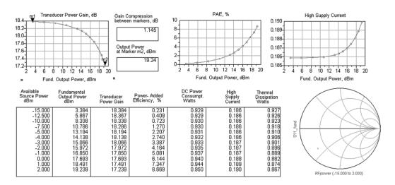
Figure 37. The two-stage amplifier performance results, with interconnect traces modeled as transmission lines.
