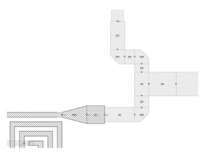
Figure 35. Part of a layout after converting traces to transmission lines
