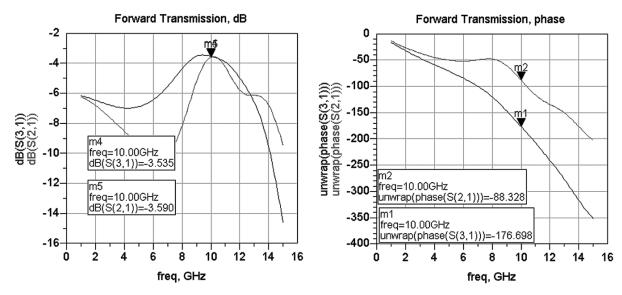
Figure 28. Optimized branch-line coupler performance
