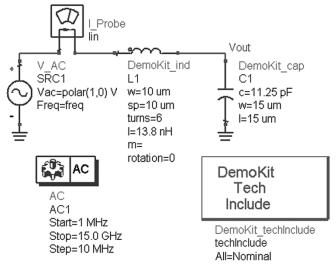
Figure 13. Simulating the impedance of a bias network
