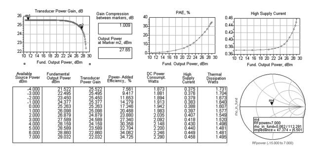
Figure 39. BalancedLumpedAmp wTLs simulation results
