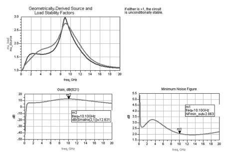
Figure 8. Gain and stability optimization results
