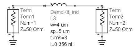
Figure 41. Simulating the S-parameters of a DemoKit inductor
