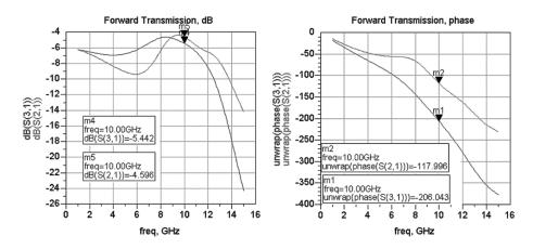
Figure 47. Momentum simulation results of the first branch-line coupler
