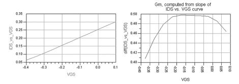
Figure 4. Plot of drain current, IDS, versus gate voltage, VGS, and transconductance, Gm.
