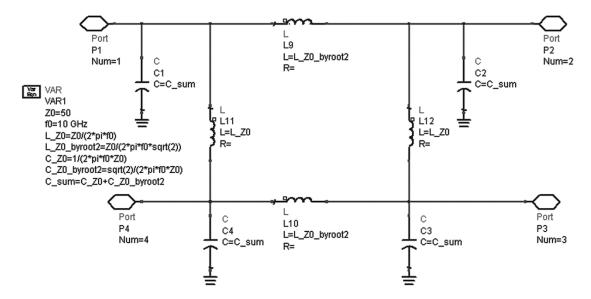
Figure 26. A branch-line coupler implemented using ideal, lumped elements
