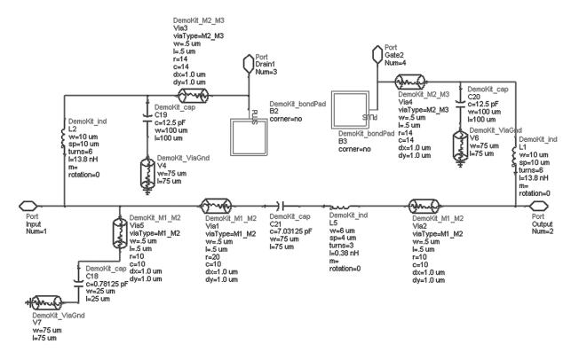
Figure 17. The interstage matching network, including design kit elements and DC bias inductors.
