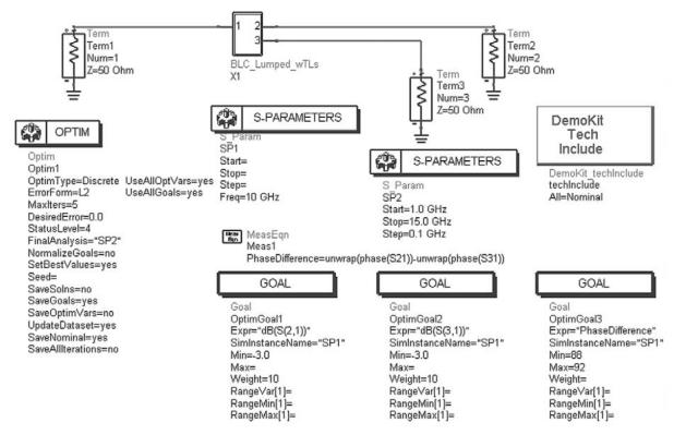
**Figure 27.** Setup for optimizing the branch-line coupler performance. The optimizable variables are defined in the subcircuit, as shown in Figure 29.
