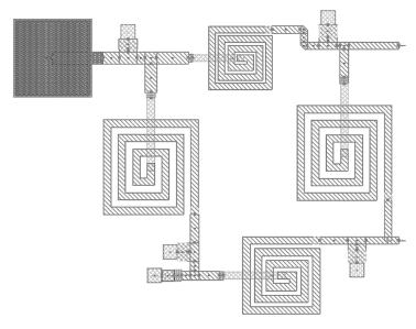
**Figure 48.** Layout of revised branch-line coupler, after optimizing inductor and capacitor parameter values, using a parameterized inductor model generated using the Advanced Model Composer.
