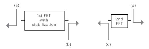
**Figure 2.** Choosing impedances. (a) Choose source Z for minimum noise figure, as long as gain remains reasonable. (b) Choose load Z for conjugate matching, after choosing source Z (although a slight mismatch was found to give a higher 1-dB gain compression output power). (c) Choose source Z for conjugate matching, after choosing load Z. (d) Choose load Z for maximum power delivered.
