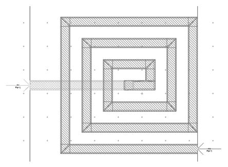
Figure 42. DemoKit inductor layout, including mesh for Momentum simulation.
