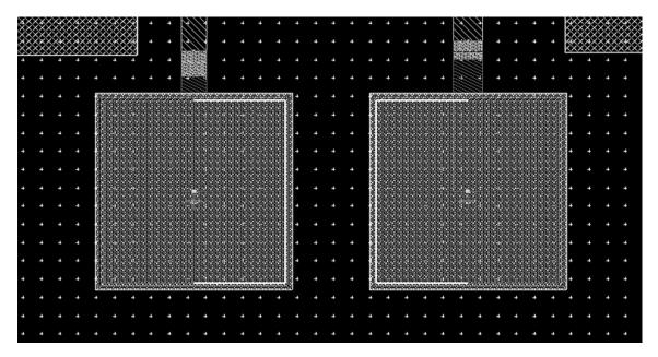
Figure B-6. A highlighted DRC error, showing two bond pads less than 100 µm apart.
