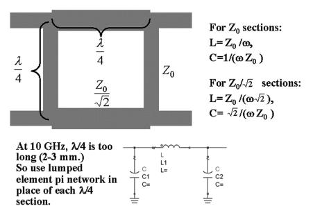
**Figure 25.** The Branch-line coupler, implemented as transmission lines, can be implemented using a  $\pi$ -network equivalent circuit for each I/4 section, using the equations shown [Reference, "Foundations for Microstrip Circuit Design," T.C. Edwards, John Wiley and Sons, 1981, pg.10.]
