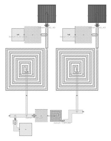
Figure 18. Interstage matching network layout
