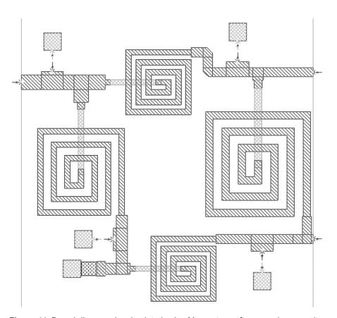
Figure 44. Branch-line coupler simulated using Momentum, after removing capacitors.
