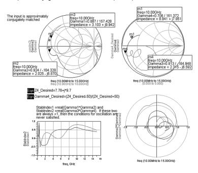
**Figure 23.** Source and load impedances close to the desired values are being generated for the second-stage device, and the stability conditions are satisfied.
