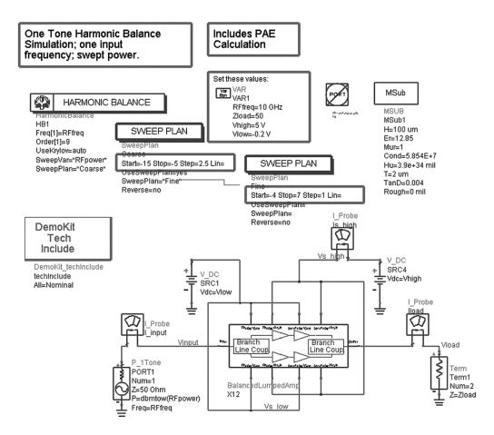
Figure 30. Simulating the gain, power, and power-added efficiency of the preliminary balanced amplifier.
