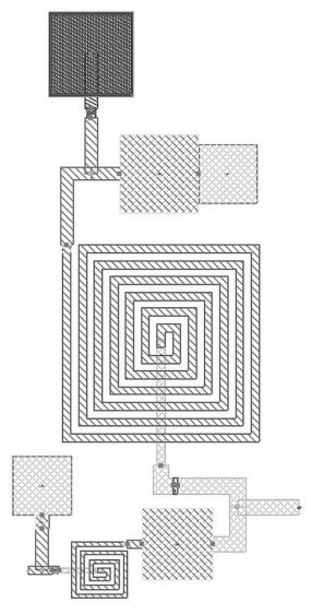
Figure 16. Corresponding input matching circuit layout, with design kit elements and a DC bias network.
