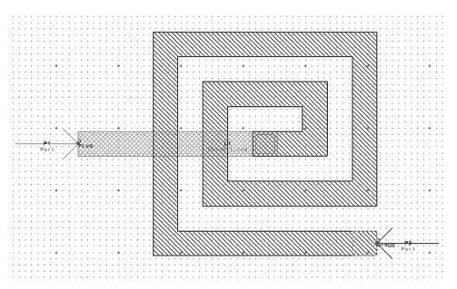
Figure A-1. A spiral inductor from the demo design kit
