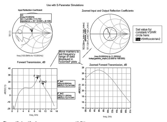
Figure 40. Amplifier frequency response near 10 GHz
