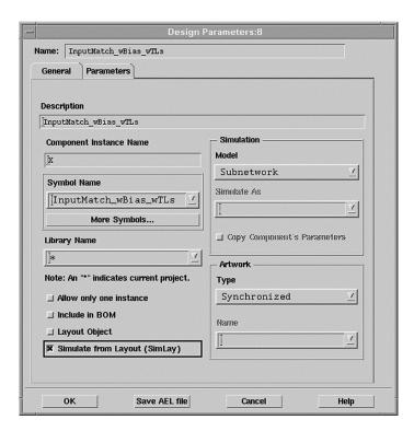
**Figure 36.** Design Parameters dialog box, allowing you to specify that the layout representation be used for the simulation.
