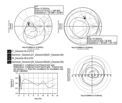
Figure 21. Source and load impedances close to the desired values are being generated by the matching networks
