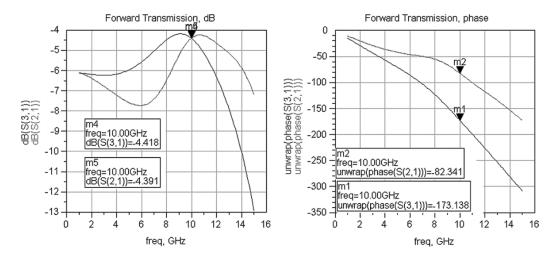
Figure 49. Simulation results of the revised branch-line coupler, after optimization.
