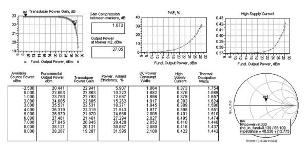
Figure 51. Performance of the balanced amplifier, including the revised branch-line coupler.
