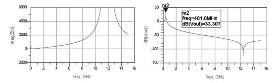
Figure 14. Bias network impedance simulation results
