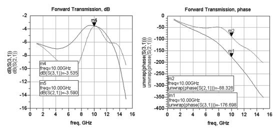
Figure 38. Branch-line coupler re-optimization results, including transmission line effects.
