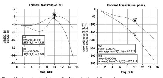
Figure 50. Momentum simulation results of the revised branch-line coupler
