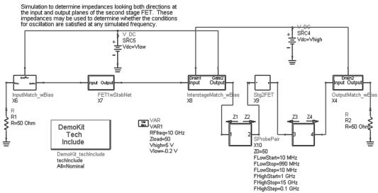
Figure 22. Two-stage amplifier output schematic
