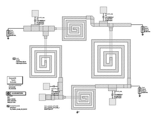
**Figure 46.** Reusing the Momentum simulation results in a circuit simulation of the branch-line coupler, which includes DemoKit capacitors.
