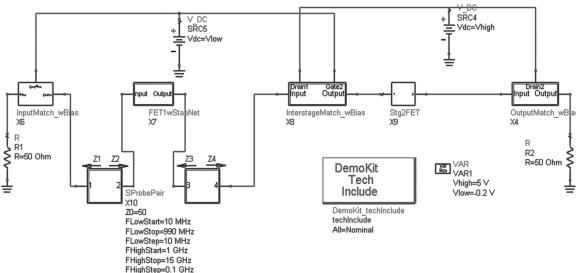
Figure 20. Determining the impedances looking both directions, at the input and output of the first stage FET.
