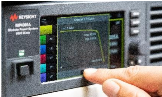
Figure 4. Intuitive touch display, setting SAS curve
