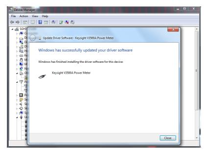
7. Go back to the **Device Manager** window. Under **Other devices** tab, repeat **Step 2** to **Step 6** for the driver installation of **'USB Serial Port'**.
