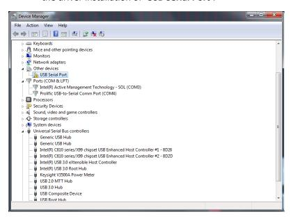
8. After all the installation have completed, the 'Keysight V3500A Power Meter' will appear under both Ports (COM & LPT) and USB controllers tabs. This indicates that the drivers are correctly installed and present.
