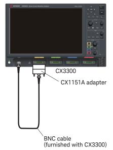
Figure 3-7 Connection Diagram for User Calibration (CX1151A)
