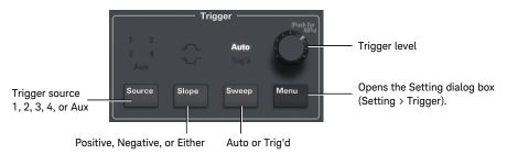
Trigger setup is shown in the Trigger summary on the summary bar which is located bottom of the screen. The summary shows the following information.
