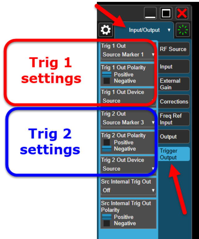
Figure 6-19 Using waveform markers to generate trigger outputs
