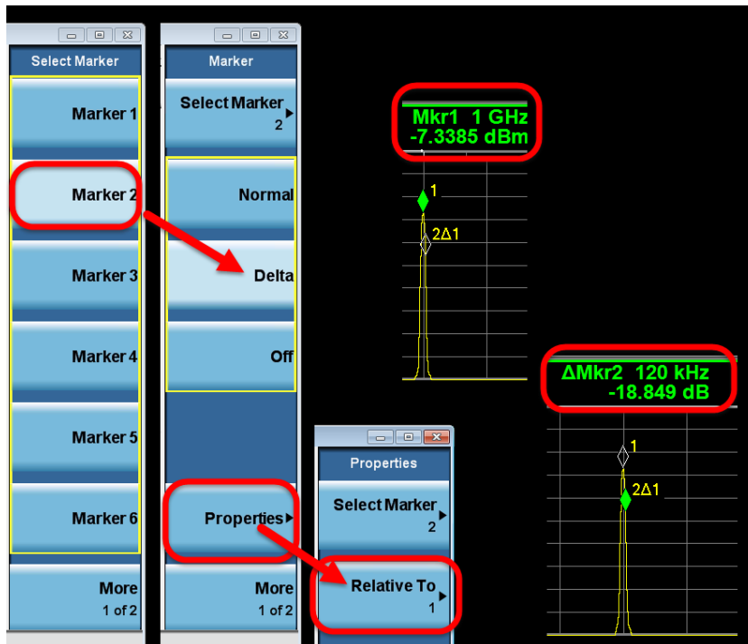
Figure 5-16 Setting up a Delta marker
