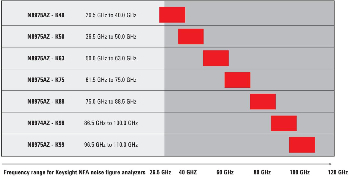
**Note:** The K-Series block downconverters can only be used with the N8975A and N9020A MXA signal analyzers.
