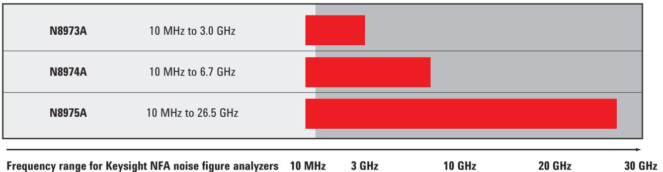
For more information on Keysight’s full portfolio of noise figure solutions see the Noise Figure Selection Guide, literature number 5989-8056EN, available at [www.keysight.com/find/nf](http://www.keysight.com/find/nf).
