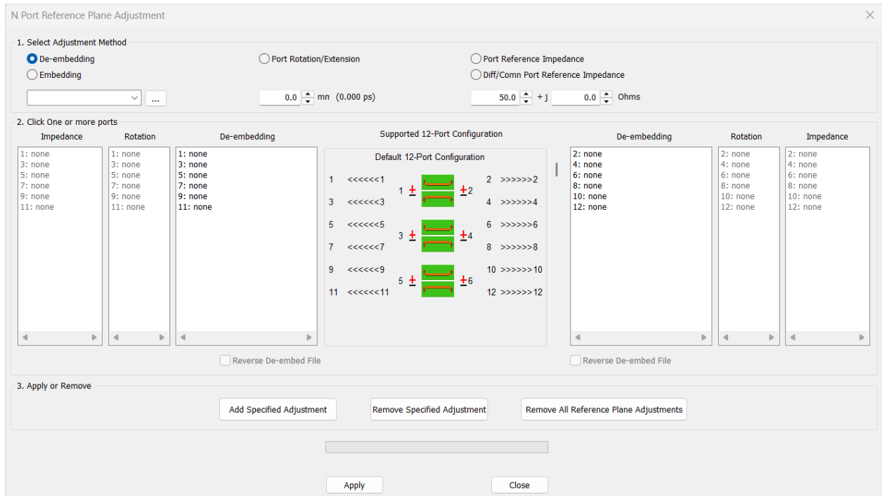
Figure 8. The effects of test fixtures can be removed from the device in post-processing through de-embedding.
