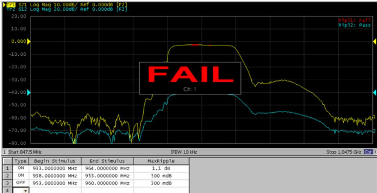
You can also specify the ON/OFF setting for the Fail Sign in the limit test menu and as well as in the bandwidth test menu. From the ripple test menu, follow the steps below to turn it ON/OFF.
