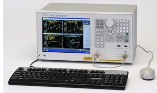
The E5063A help provides an easy access to the information related to the use of Agilent E5063A Network Analyzer. Pressing **Help** key on the front panel displays the topic related to the selected softkey.
