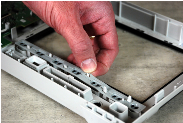
Figure 51 Remove the softkey keypad from the bezel
