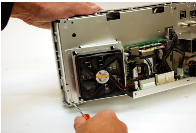
Figure 30 Removing the bottom left rear deck screw
