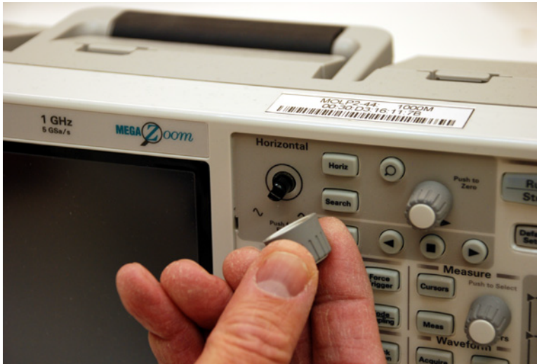
Figure 21 Removing the front panel knobs
