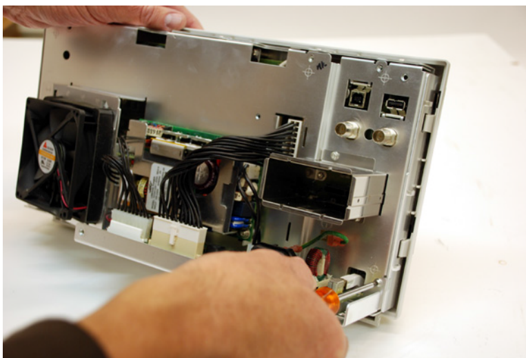
Figure 29 Removing the bottom right rear deck screw
