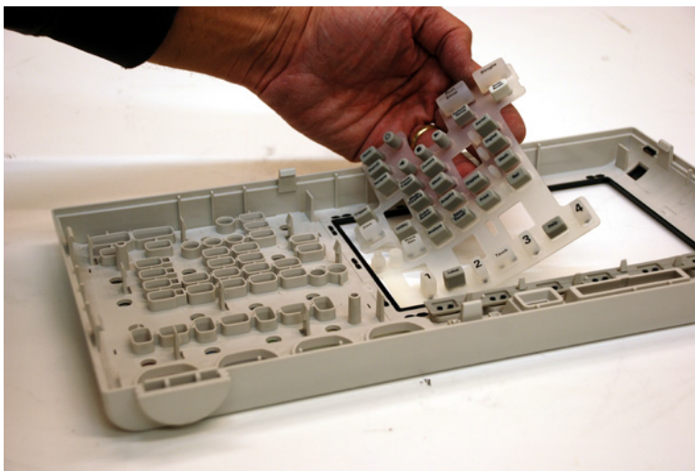
Figure 53 Remove the keyboard keypad from the bezel
