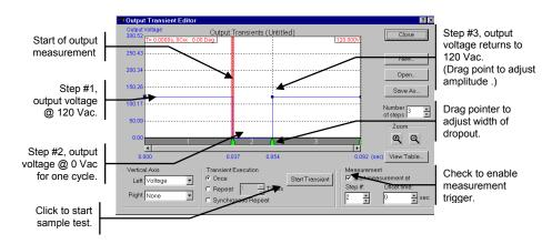
You can use the transient editor to make any final adjustments to the ac line dropout test such as fine tuning the width of the dropout, or positioning and enabling the measurement trigger.
