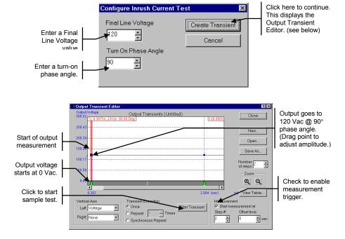
You can use the transient editor to make any final adjustments to the inrush current measurement such as fine tuning the width of the transient step, or positioning and enabling the measurement trigger.
