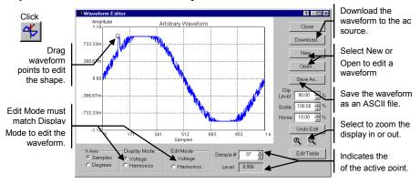
To create or edit waveforms in the harmonic format, set the Edit Mode and the Display Mode to **Harmonics**. Note that continually switching edit modes will result in cumulative waveform truncation errors. Therefore, select only one edit mode to work in. Switching display modes does not cause recalculation errors.
