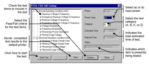
To configure the Test Pass/Fail criteria of the RTCA/DO-160 tests, click **Options**. You can specify either ac input or dc input tests. Note that both Pass/Fail criteria must be true for the ac or dc input tests to pass.
