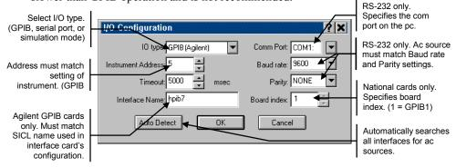
If there seems to be no communication between the Agilent AC Source GUI and the ac source, select **Auto Detect** to detect any ac sources connected to your pc. Also try resetting the I/O interface by clicking the red reset button. This also resets the ac source to its default settings.
