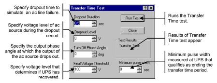
The transfer time results appear in the Test Results area of the dialog box. The transfer time is displayed in seconds. When you close the Transfer Time Test dialog box, you will be able to see both the output of the ac source and the output of the UPS in the waveform display area.
