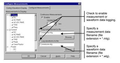
The measurement data file saves measurements in a comma-separated table of values. The columns in the list correspond to all available measurements, with blanks for non-measured values. For 3-phase units, only information from the selected phase will be saved.
