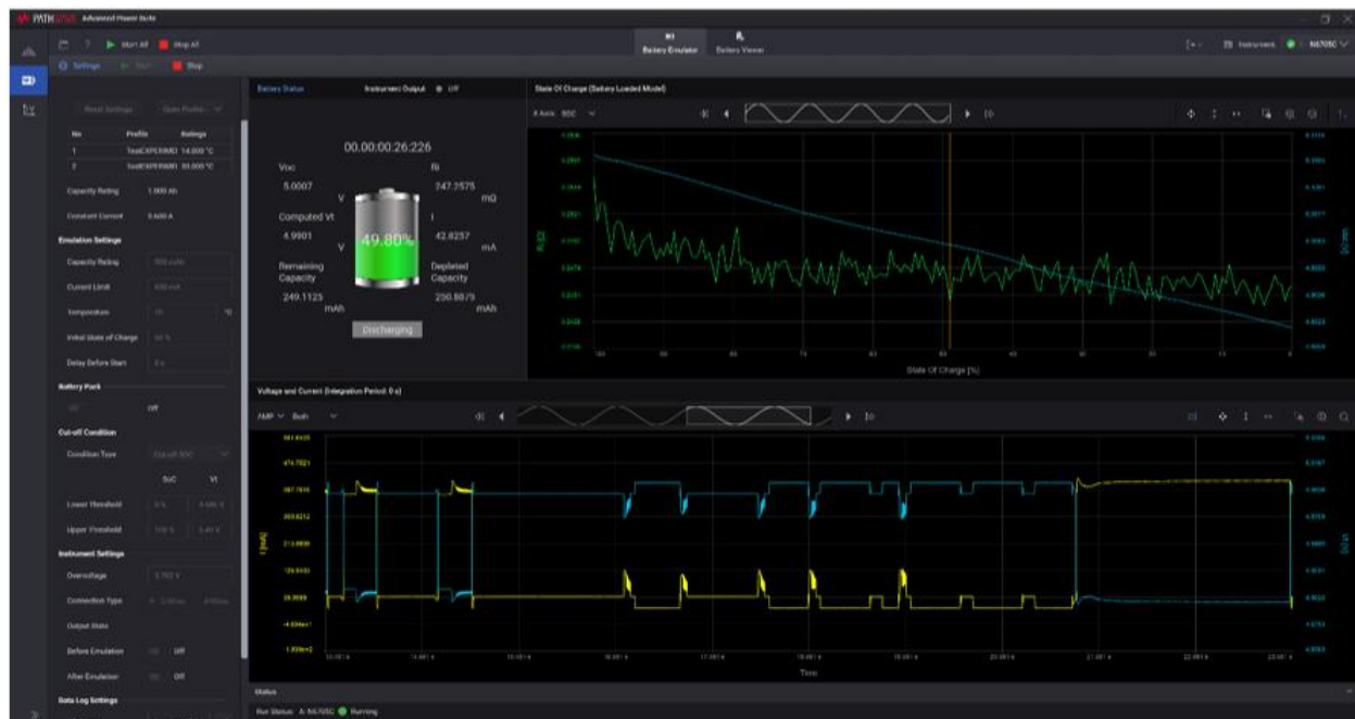
Figure 6. PW9253A Emulating multiple battery models at different temperatures.
