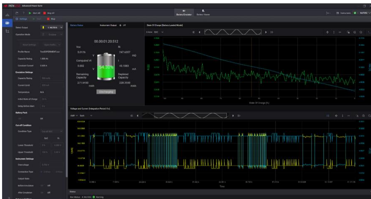
Figure 5. PW9253A Emulating Lithium battery powering a low-power device.
