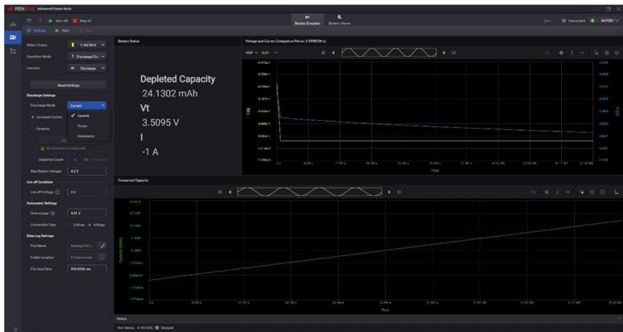
Figure 9. PW9253A enables you to choose various discharge mode options (constant current, power, resistance, and dynamic current discharge)
