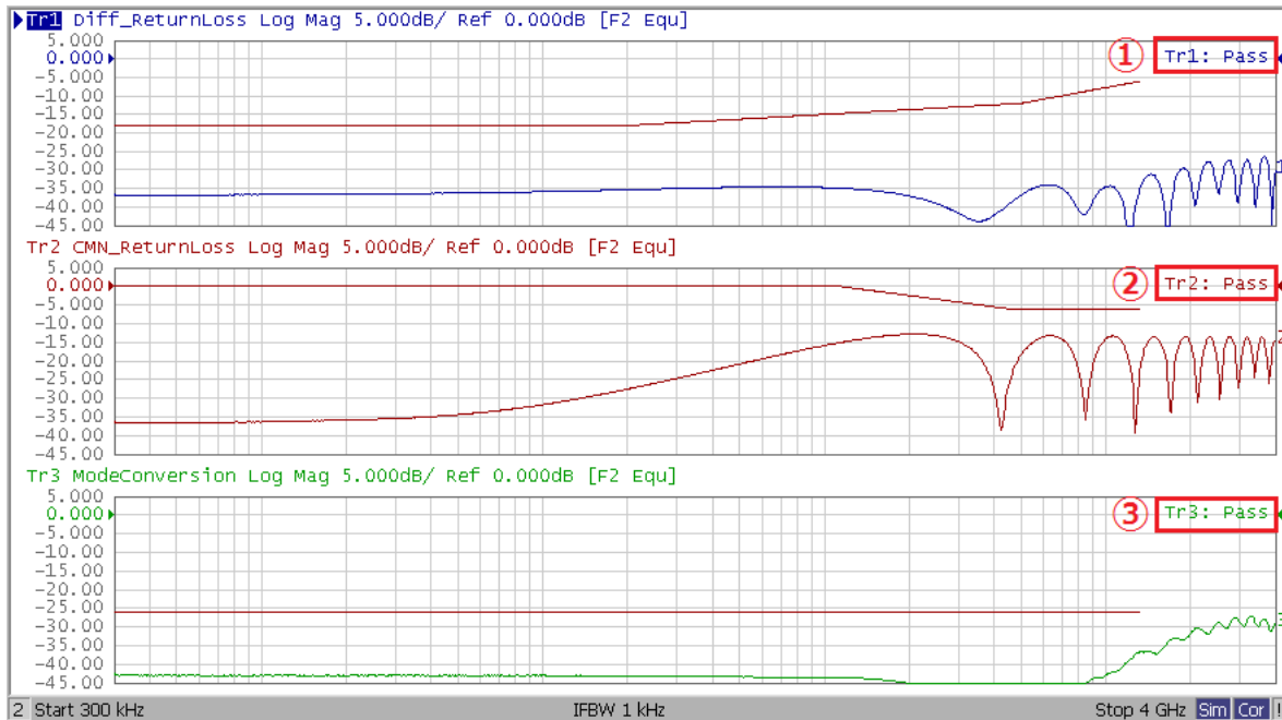
Figure 5-3 Differential Return Loss, Common-Mode Return Loss and Mode Conversion Limits (HS-RX) Example
