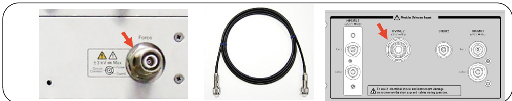
Figure A2-4. Breakdown of the cable connection for 20 A configuration.
