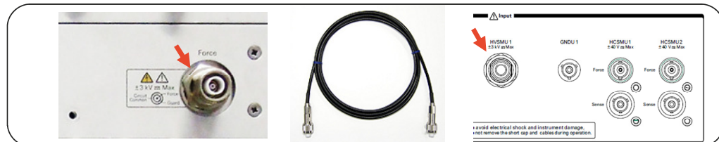
Figure 2-10. Breakdown of the cable connection for 40 A configuration .
