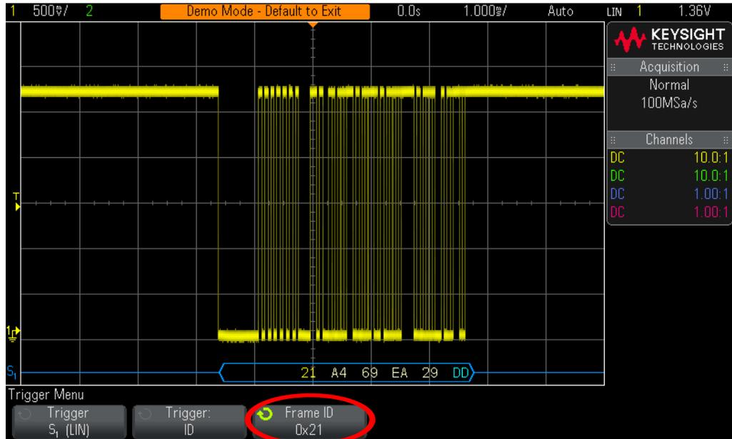
**Figure 75** While triggering on LIN frame = 21<sub>HEX</sub>, the scope’s hardware-based decoding reveals parity bit errors in the frame ID field.
