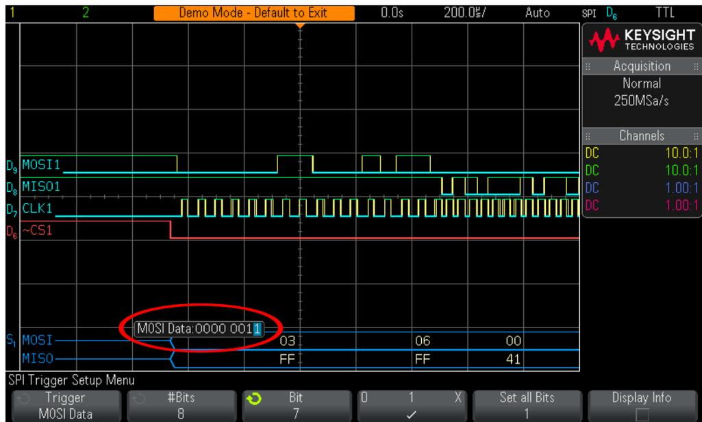
**Figure 57** Triggering on MOSI data = 03<sub>HEX</sub>.
