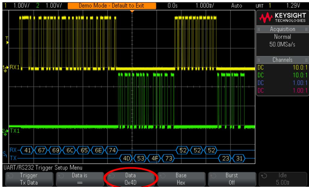
**Figure 62** Triggering on Tx = 4D<sub>HEX</sub>.
