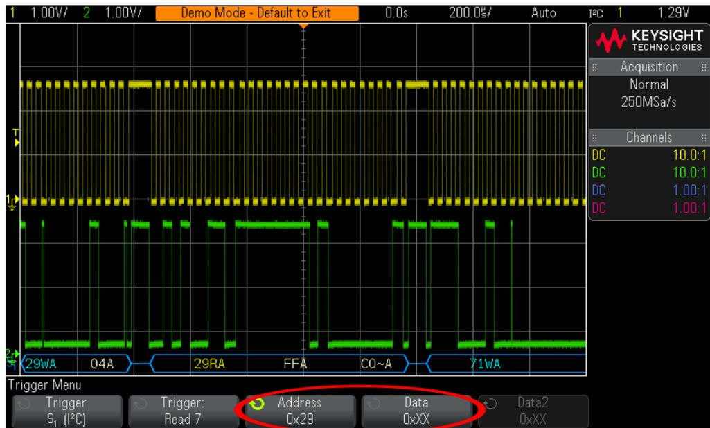
**Figure 52** Triggering on I<sup>2</sup>C traffic.
