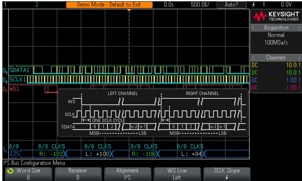
**Figure 80** Decoding I<sup>2</sup>S signals.
