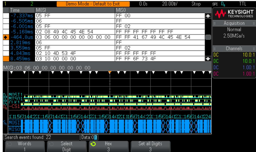
**Figure 58** Automatic Search & Navigation on SPI traffic.
