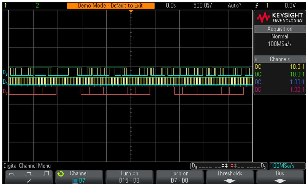
**Figure 79** Capturing I<sup>2</sup>S signals using the scope's digital channels of acquisition (MSO).
