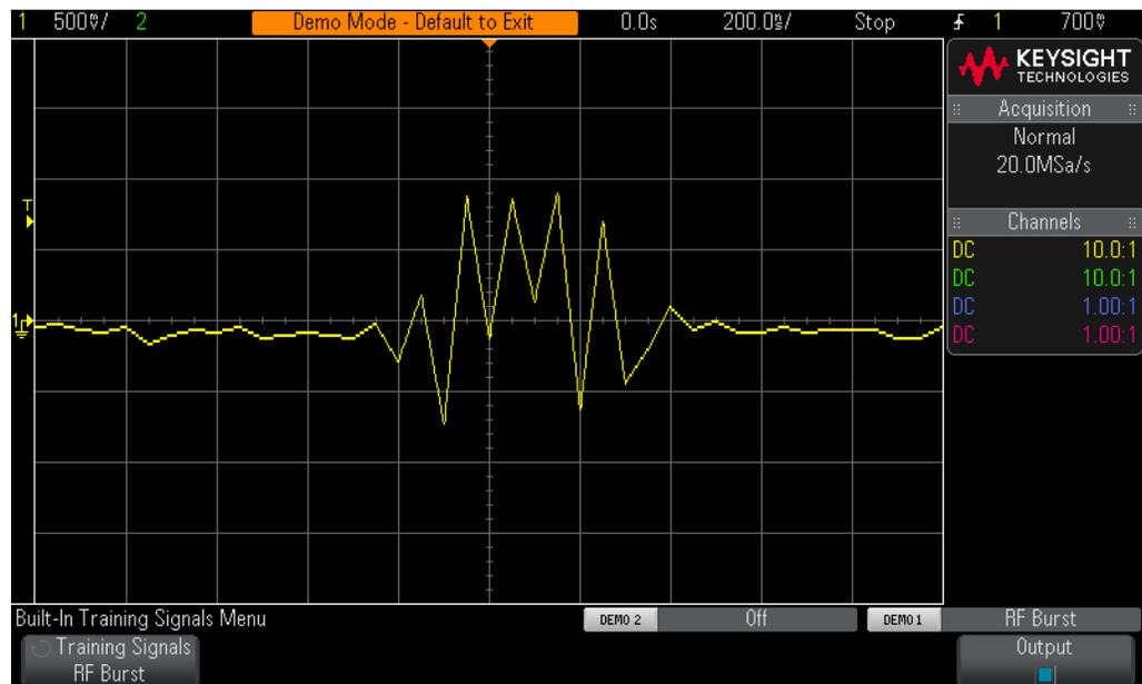
**Figure 17** Zooming in reveals an under-sampled waveform.
