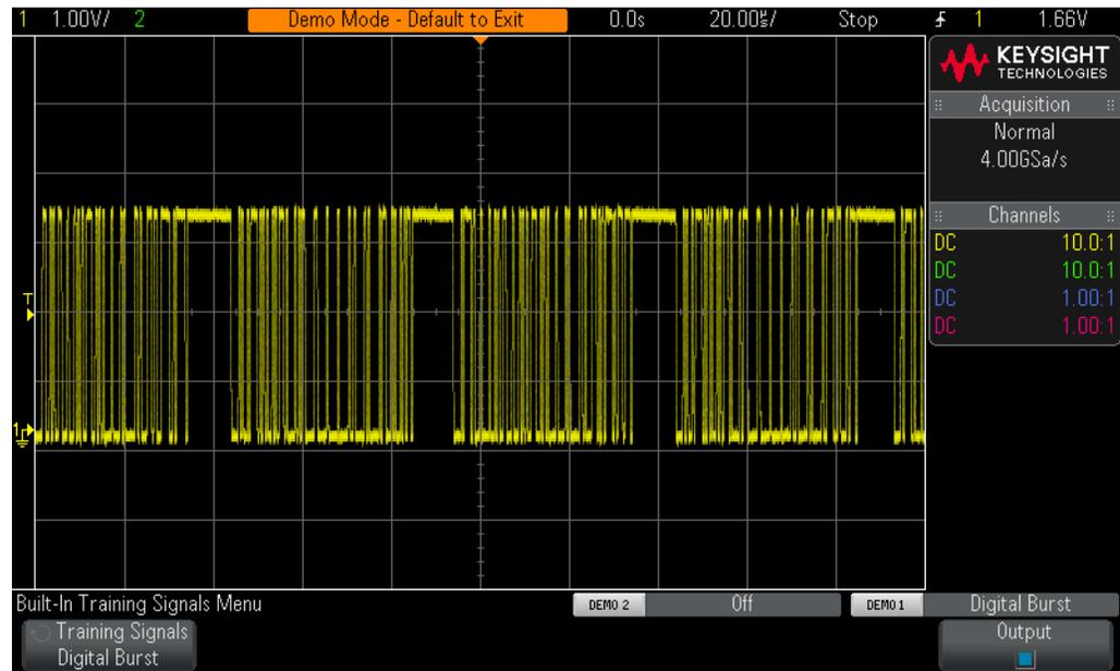
**Figure 23** Single-shot acquisition reveals digital burst activity.
