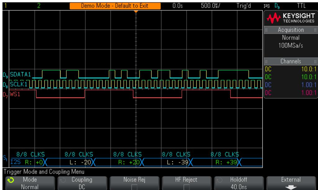
**Figure 81** Triggering on I<sup>2</sup>S right-channel = +20.
