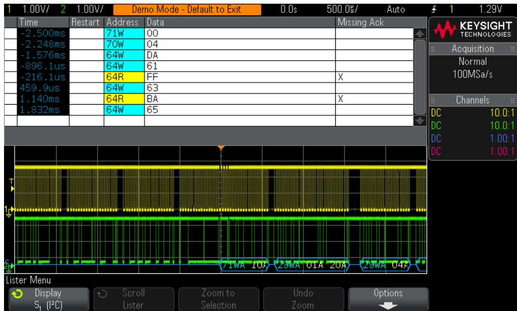
**Figure 51** Decoding I<sup>2</sup>C serial bus traffic.
