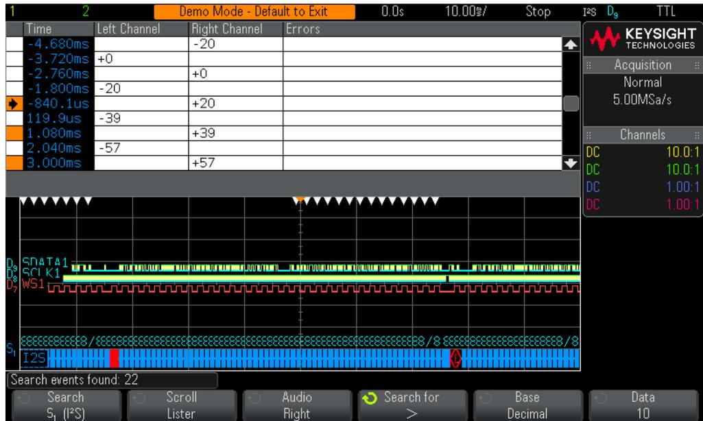
**Figure 82** Automatic Search & Navigation on I<sup>2</sup>S data.
