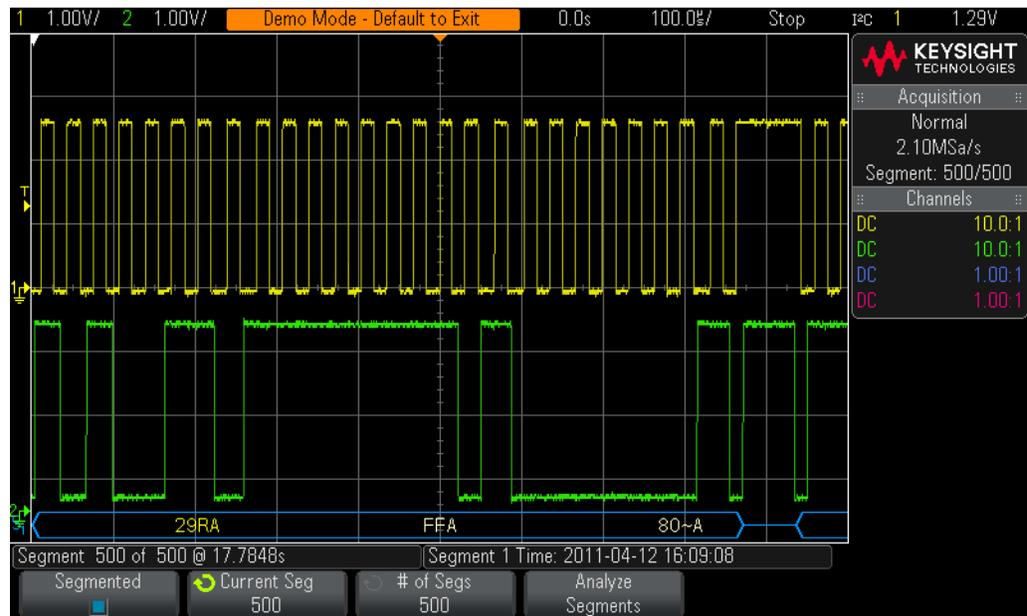
**Figure 54** Using the scope's Segmented Memory acquisition to selectively capture more I<sup>2</sup>C traffic.
