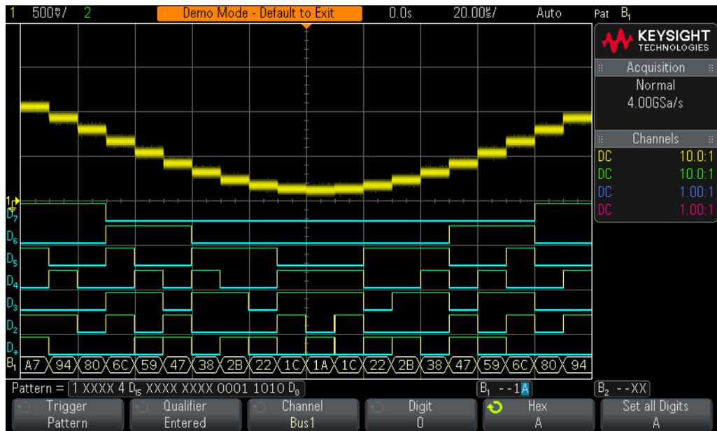
**Figure 49** Triggering on pattern = 1A<sub>HEX</sub>.
