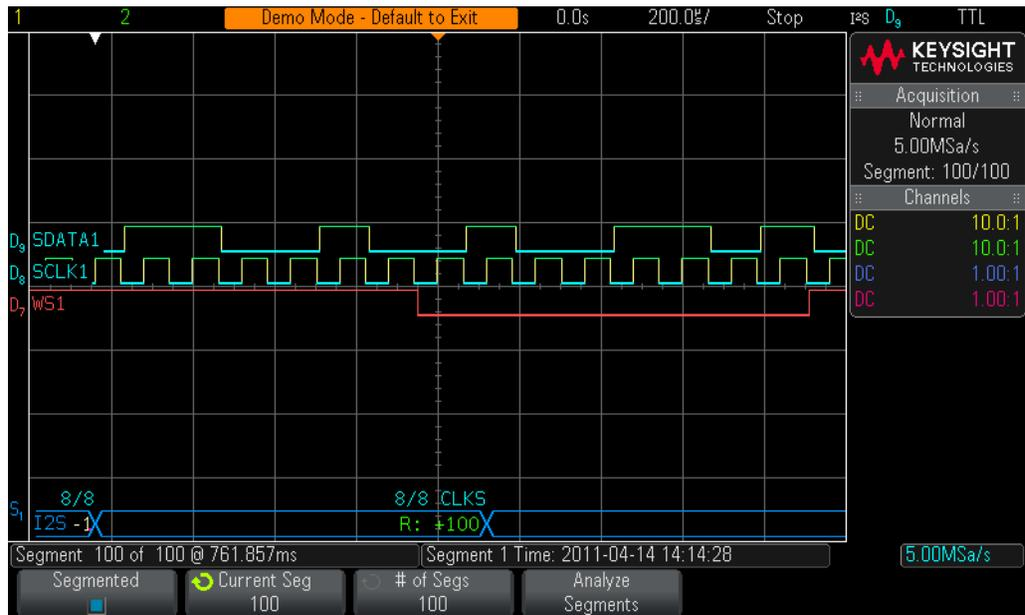
**Figure 83** Using the scope's Segmented Memory acquisition to selectively capture more I<sup>2</sup>S traffic.
