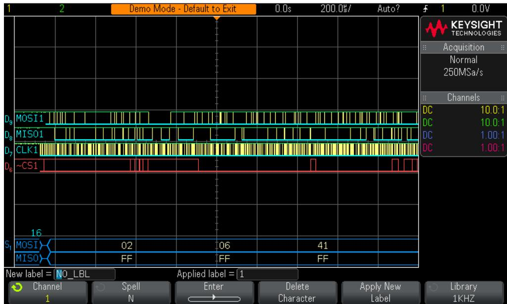
**Figure 56** Decoding a 4-wire SPI serial bus.
