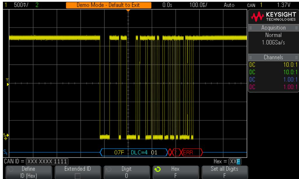
**Figure 69** While triggering on CAN data frame = 07F<sub>HEX</sub>, the scope’s hardware-based decoding reveals infrequent error conditions.
