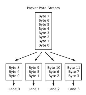
The previous example shows data striped in bytes, but it can also be striped in byte pairs or other data lengths.
