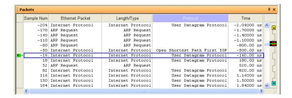
In the Packet Viewer window, you can insert or delete columns as desired (see "To insert or delete packet decode columns" (in the online help)).
