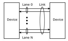
The number of serial channels in a link are sometimes described with a number and an "x". For example, InfiniBand can have 1X, 4X, and 12X links; PCI Express can have x1, x2, x4, x8, and x16 links.
