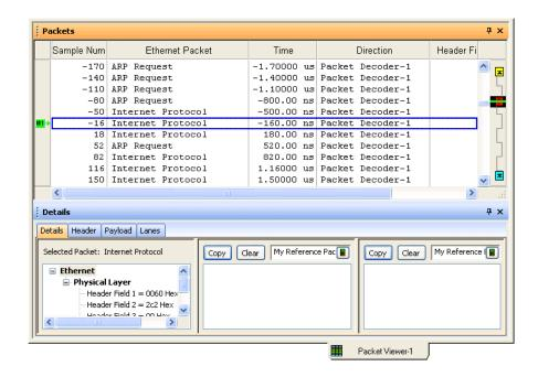
You can color-code packet types in the Packet Viewer window and add descriptive tool tips with <PacketDisplay> elements inside the <PacketType> elements (see "Describing Packet Type Colors" on page 47).
