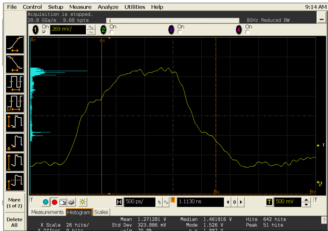
Figure 14 V_{OH(AC)} Test - Maximum AC Output Logic High in Infiniium oscilloscope.
