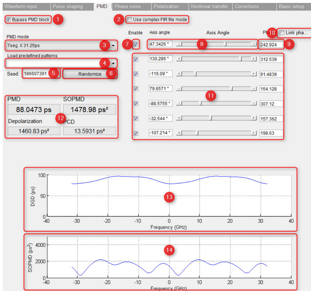
Figure 39 PMD tab (Concatenation of birefringent segments)
