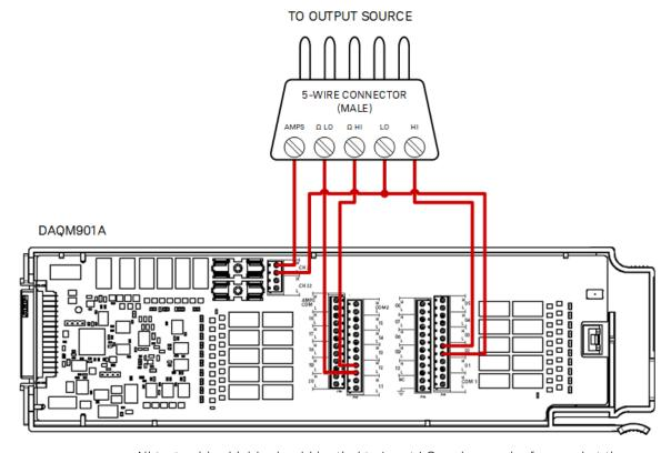
All test cable shields should be tied to Input LO and ground referenced at the calibrator's output terminals. This configuration is recommended for noise reduction and settling time performance during calibration.
