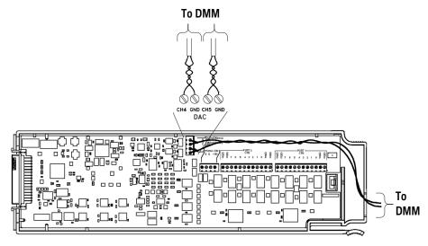
**2** For each analog output, set each output value in the table below. Compare the measurement results to the appropriate test limits shown in the table below.
