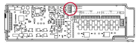
A wire is not needed to short Channel 04 GND to Channel 05 GND because they are already shorted on board.
