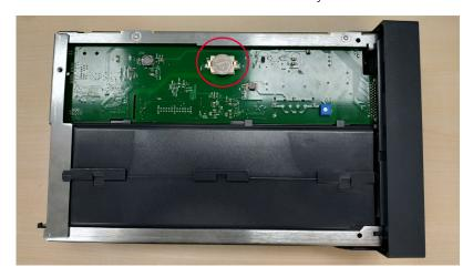
4 Measure the battery voltage using an external DMM.
