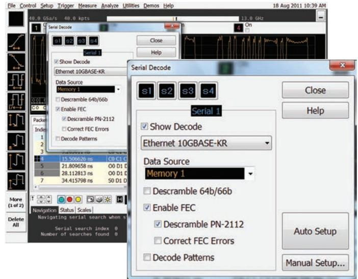
Figure 2. The 64b/66b and link training setup menu includes an “Auto Setup” tab, which enables you to begin decoding 10Gbase-KR signals in less than 30 seconds.
