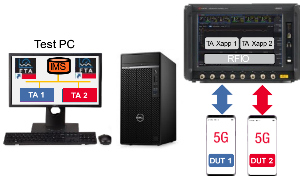
Figure 21. Functional tests performed on two UEs with one UXM 5G
