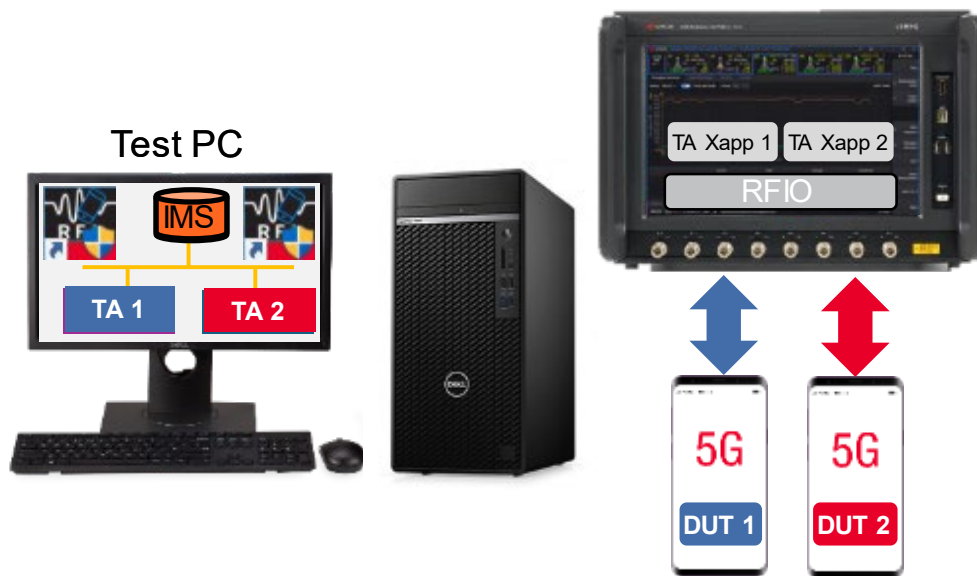
Figure 20. RF performance of two UEs verified with one UXM 5G
