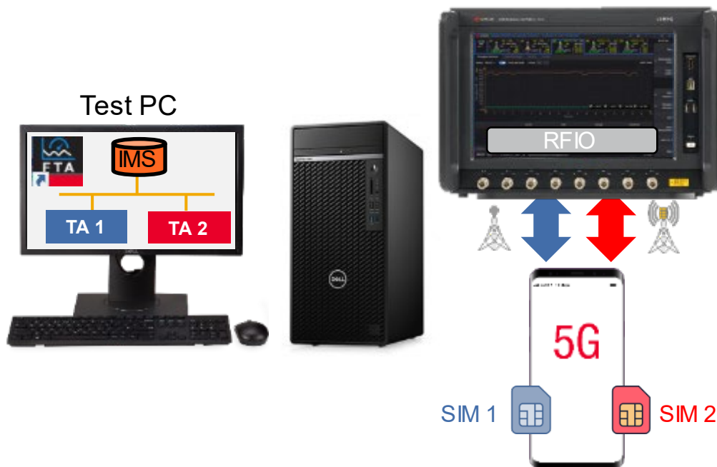
Figure 19. Dual-SIM UEs tested with one UXM 5G
