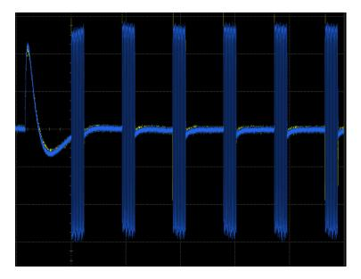
There is a chance that the application detecting the OOB signal if some OOB stream portion does not have the spike shown above. If this is the case, the tester should try to re-run the test again.
