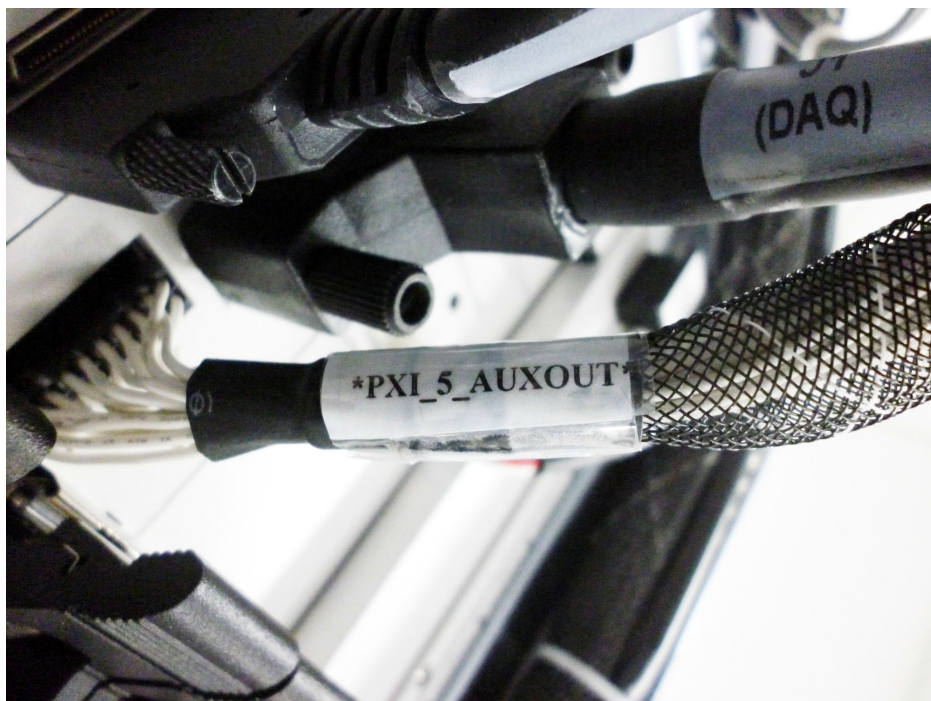
Figure 1-16 Interface cable label example (*PXI_5_AUXOUT*)
