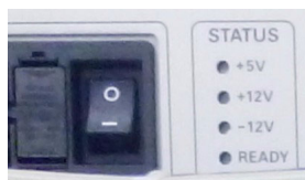
Figure 1-19 TS-8989 system power switch (instrument interface view)
