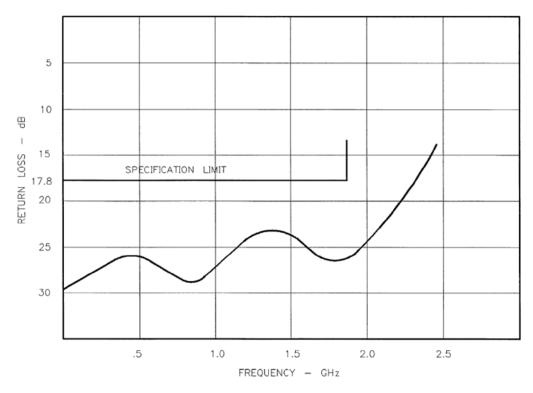
Figure 2 Typical return loss versus frequency
