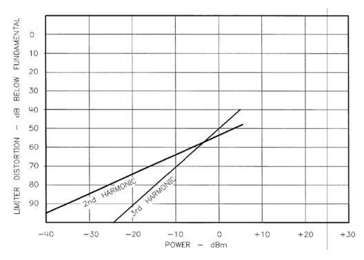
Figure 4 Typical harmonic distortion versus input power
