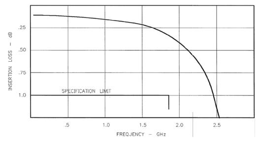
Figure 1 Typical insertion loss versus frequency
