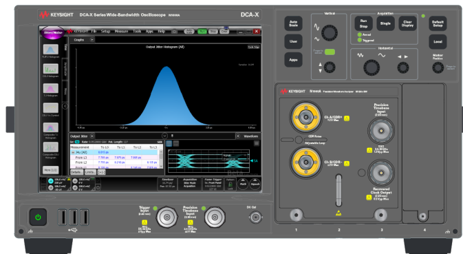
Figure 1. N1000A with Installed Module
