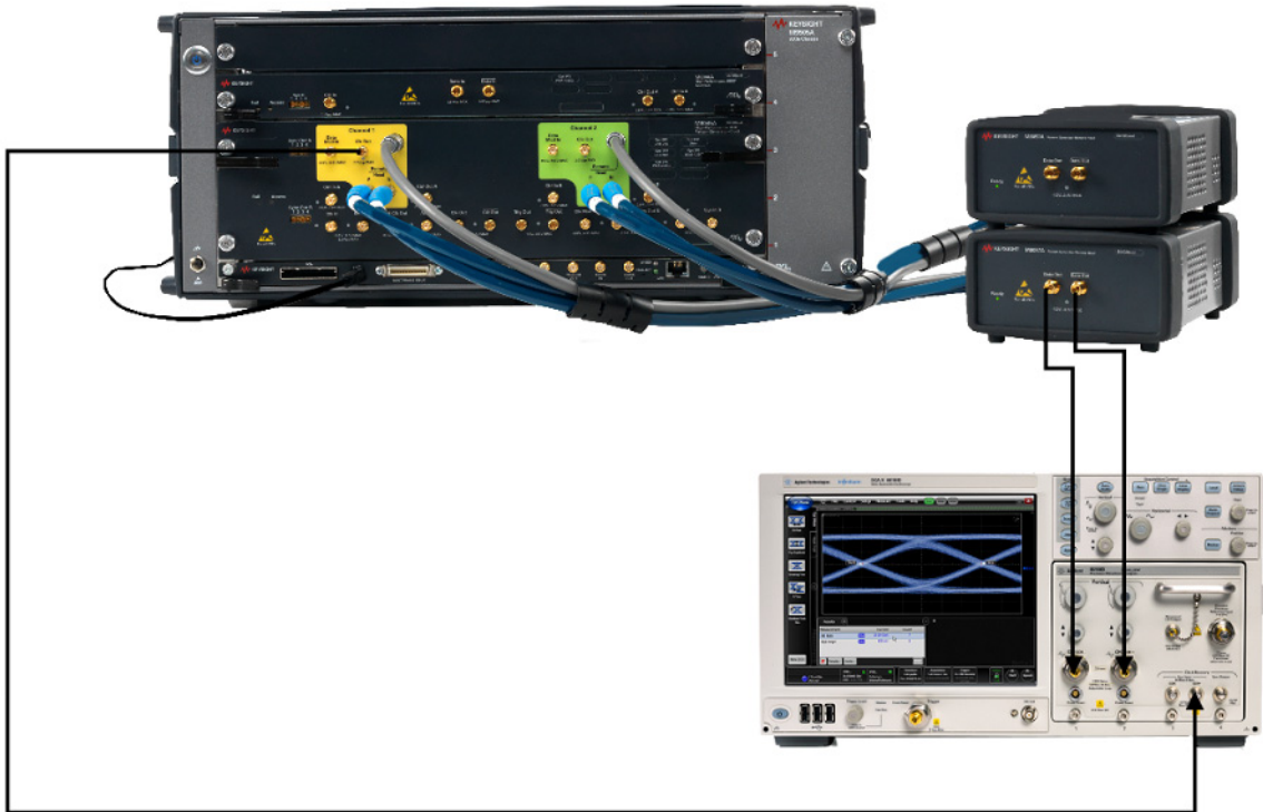
Figure 24 SJ Calibration connections for C2M Host & C2M Module
