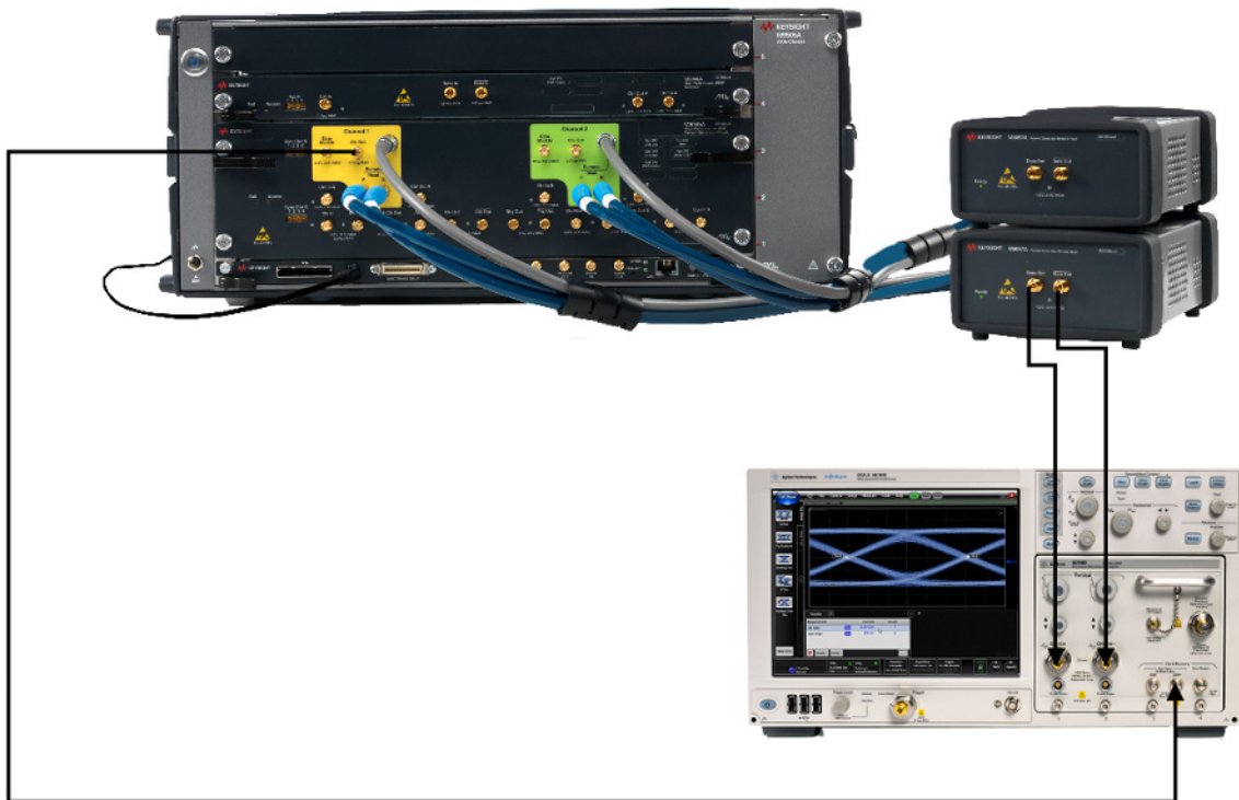
Figure 23 JRMS Calibration connections for C2M Host & C2M Module
