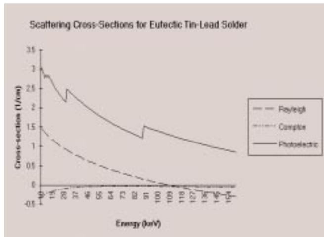
Fig. 1. Scattering cross-sections for eutectic tin-lead solder versus energy. The ordinate is on a  $\log_{10}$  scale. Note the dominance of the photoelectric cross-section, followed by the Rayleigh and Compton cross-sections.
