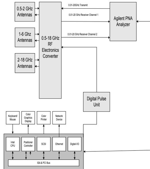
**Figure 2 – Cheetah Radar System**
