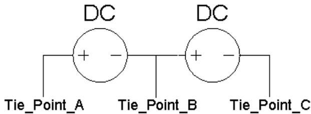
5. Select Tasks, Design Fixture, Change Wires. Enter the power supply node name under Node, the appropriate phantom nodes entered in step 4, the BRC's of the supplies you are using, and ground (assuming one side of one supply connects to ground, if not, enter the name of the second node being used.)
