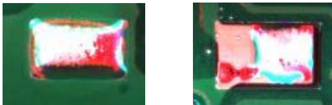
Figure 3. Solder Pad coverage. Photo to the left tin-lead solder, to the right lead-free
