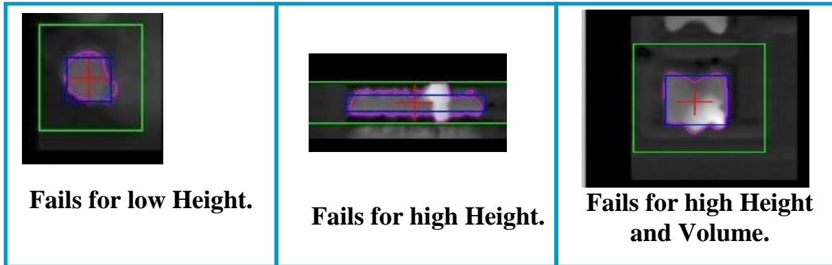
Figure 3: A few examples of defects only detectable with 3D SPI.
