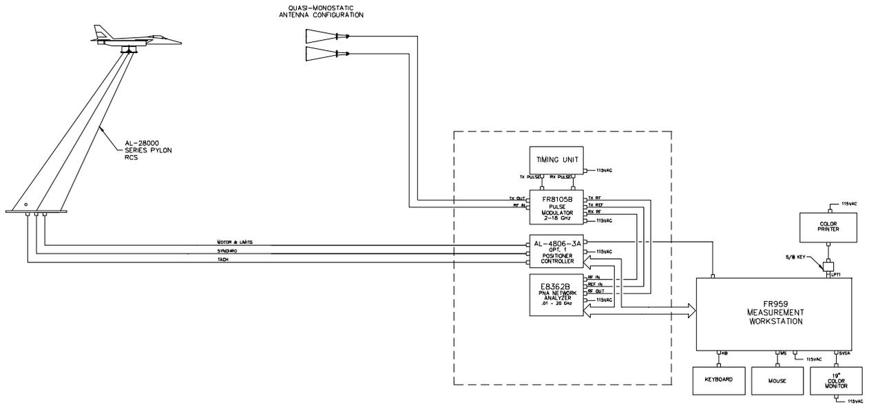
Figure 1 Block Diagram of High Speed *StingRay* Gated-CW Instrumentation Radar (2-18 GHz)
