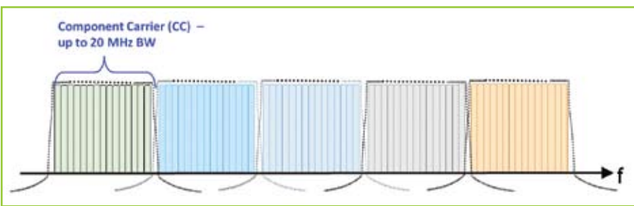
Figure 1. Aggregation of contiguous component carriers.
