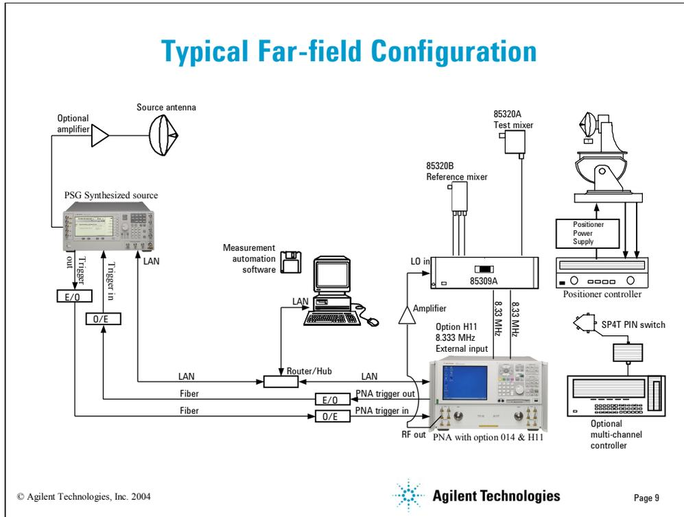
The configuration for a PNA in a far-field antenna configuration is as shown here:
