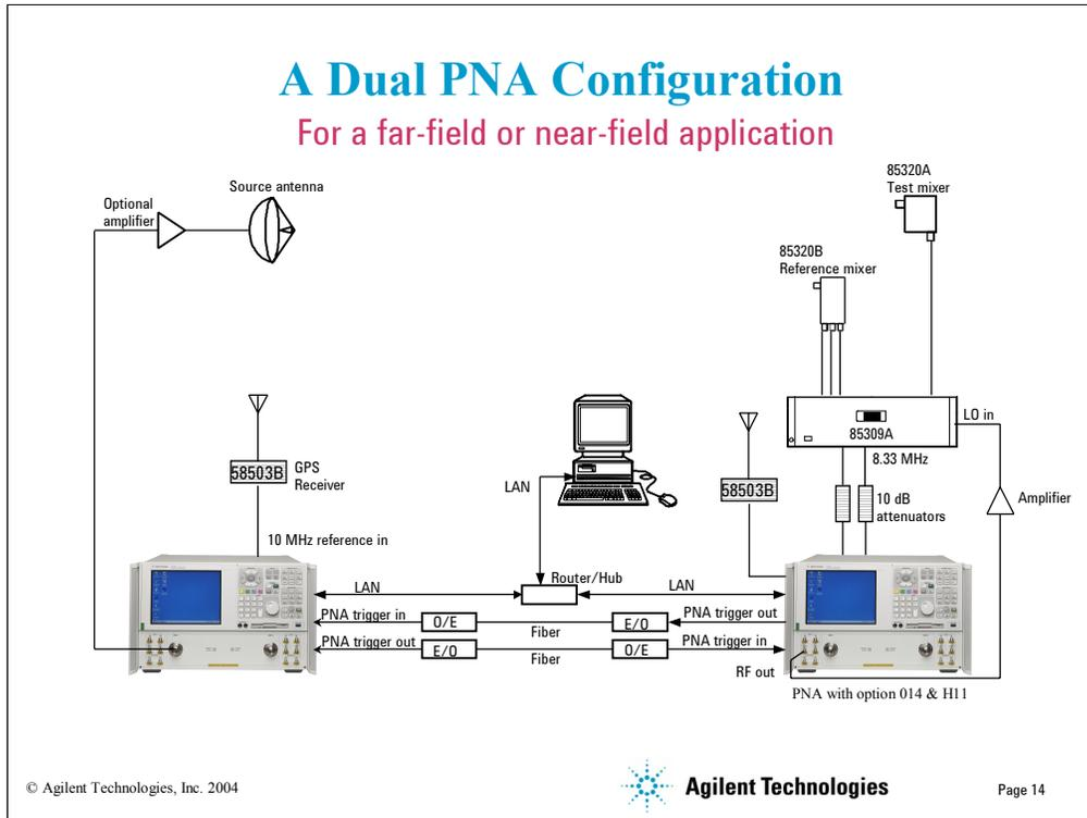
Shown here is a concept that has not been fully verified by Agilent Technologies, but holds good promise for applications which would require extremely fast frequency stepping capability.
