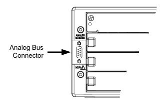
To avoid electrical shock due to high voltages present on the Analog Buses, the software requires that all modules not under test be disconnected from the Analog Buses. With the verification terminal block connected to an installed module, all voltages present on the Analog Buses will also be present on the terminal block's D-Sub connector (located at the end of the ribbon cable).
