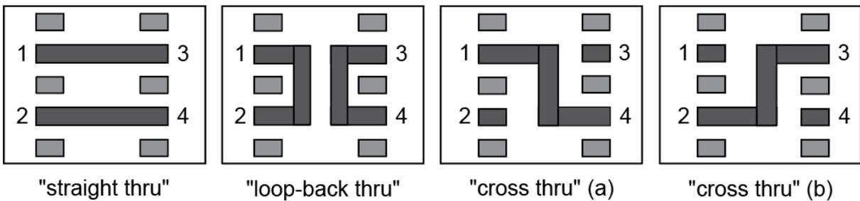
**Figure 4.** Examples of common thru configurations of a GSGSG probe.
