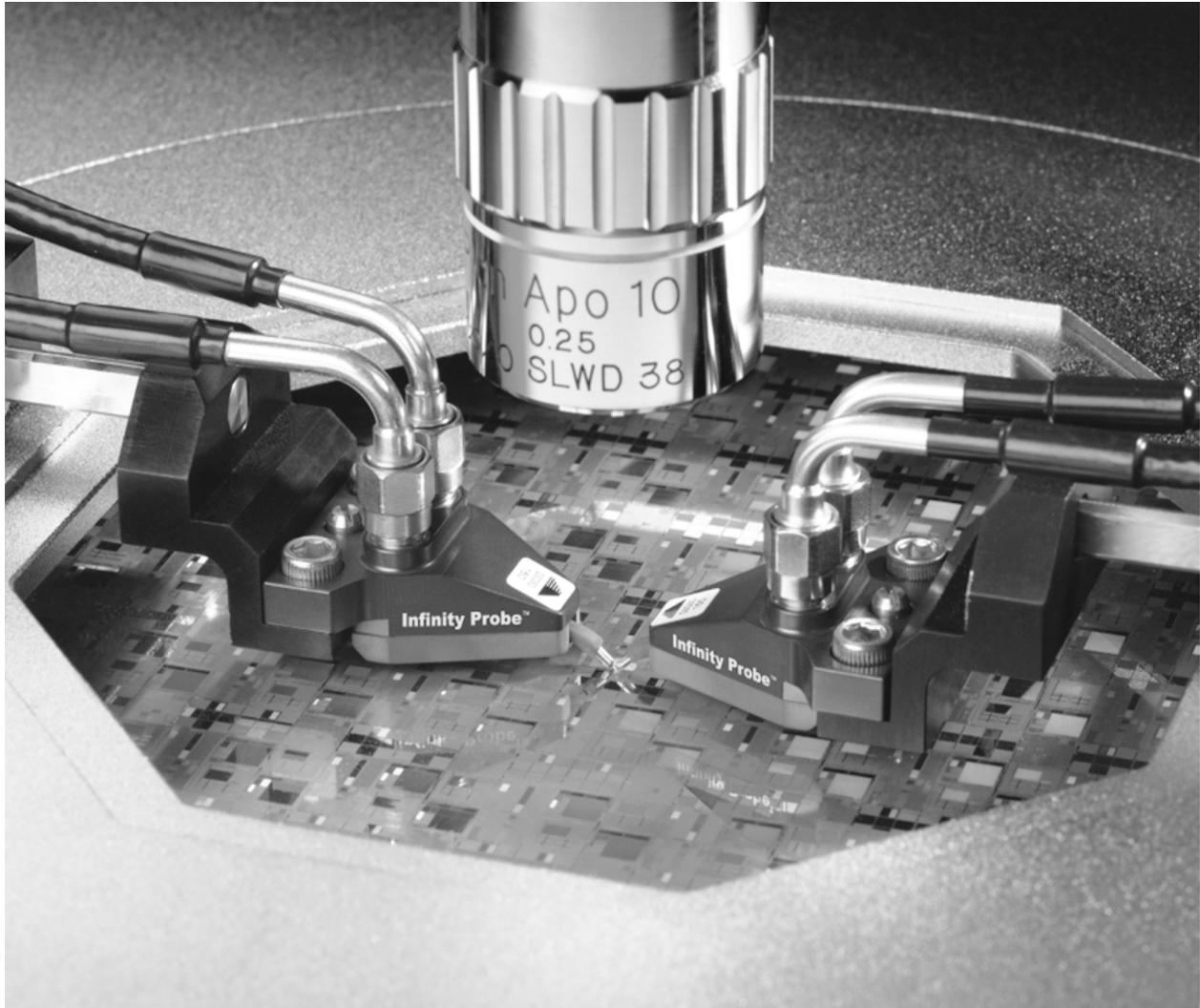
**Figure 2.** Dual line Infinity probe from Cascade Microtech. Available in GSGSG and GSSG configurations with pitches 100, 125, 150, 200, 225, and 250  $\mu\text{m}$ . For more details, please contact Cascade Microtech at [www.cmicro.com](http://www.cmicro.com)
