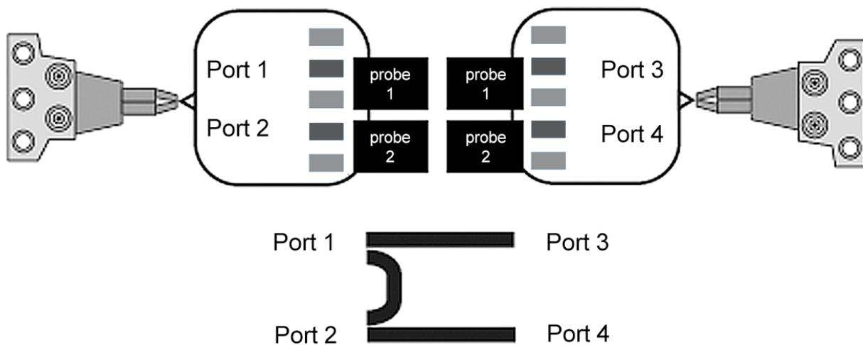
**Figure 6a.** Assigning test ports as either probe 1 or probe 2 offers the PNA-L the most efficient way of executing minimum thru. This example allows the PNA-L to maximize the number of straight thrus and minimize the number of non-straight ones.
