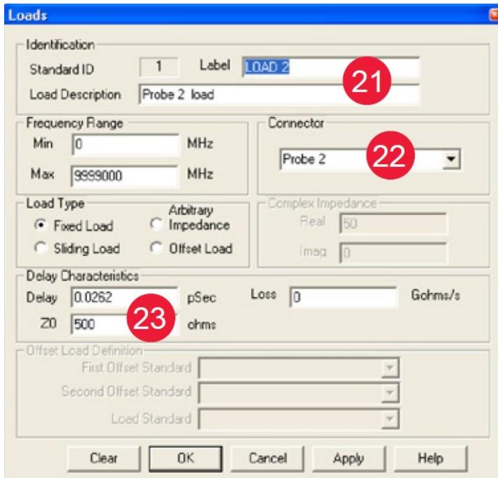
**Figure 9b.** Changing to “LOAD 2” and “Probe 2”.
