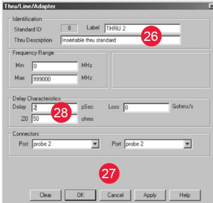
**Figure 10b.** Changing to "THRU 2" and "probe 2".
