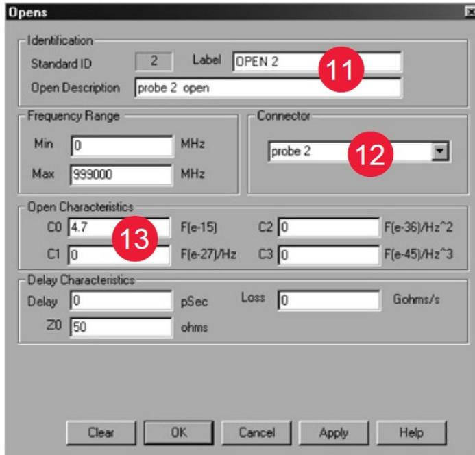
**Figure 7b.** Changing to "OPEN 2" and "probe 2".
