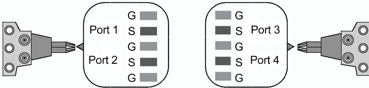
**Figure 3.** Port assignment used in this application note: ports 1 and 2 on the left, ports 3 and 4 on the right.
