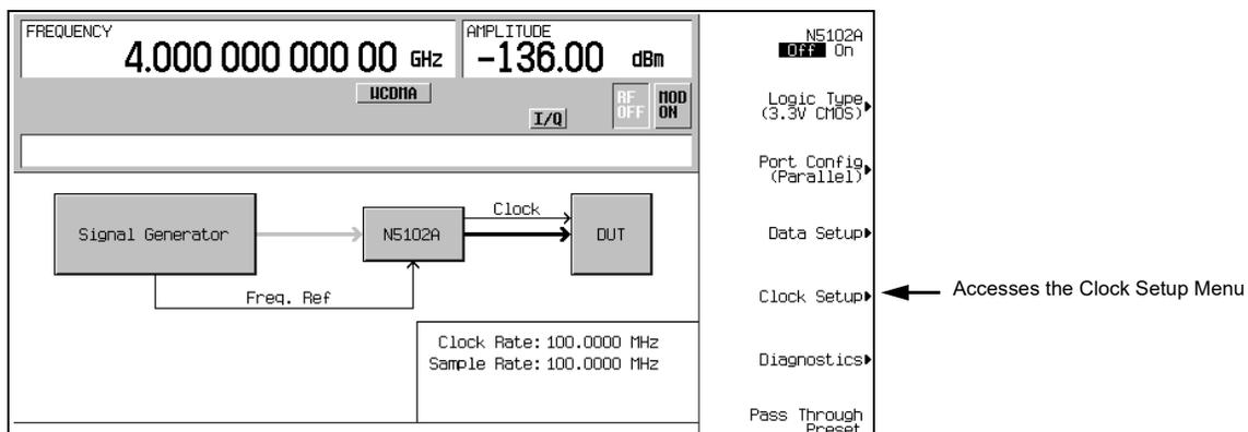
From this softkey menu, set all of the clock parameters that synchronize the clocks between the N5102A module and the PSG. You can also change the clock signal phase so the clock occurs during the valid portion of the data. **Figure 12-14** shows the clock setup menu.
