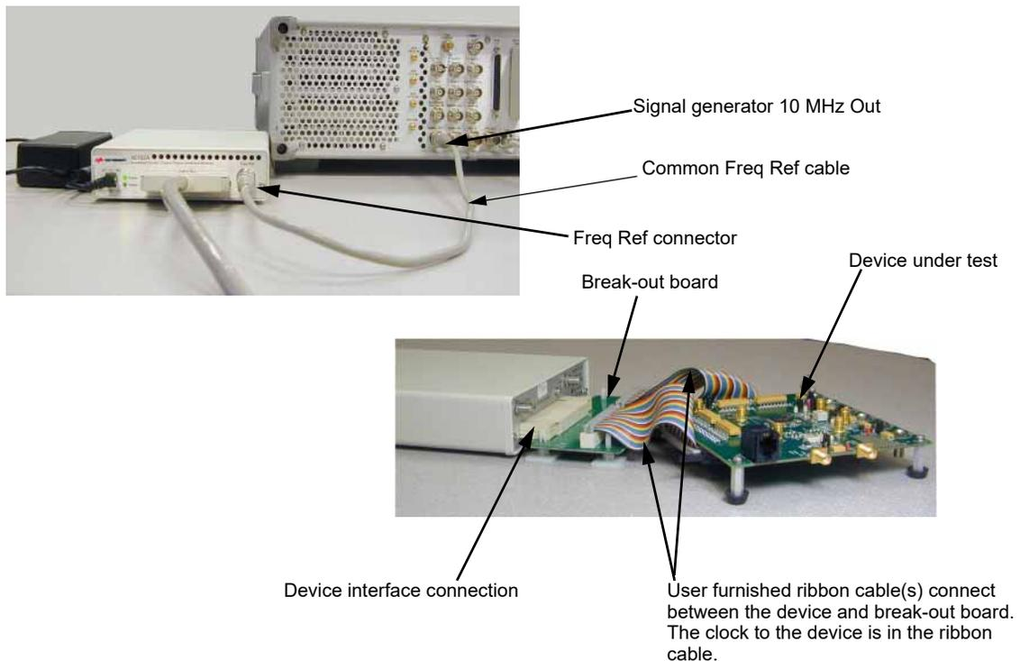
1. Refer to the five setup diagrams in [Figure 12-3 on page 295](#) and connect the frequency reference cable according to the clock source.
