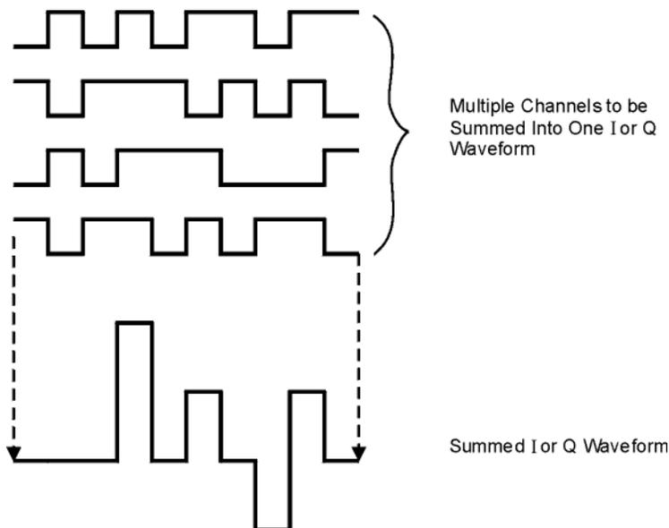
The I and Q waveforms combine in the I/Q modulator to create an RF waveform. The magnitude of the RF envelope is determined by the equation  $\sqrt{I^2+Q^2}$ , where the squaring of I and Q always results in a positive value.
