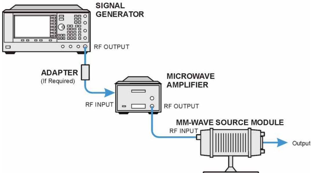
**Figure 12-24** Setup for E8267D PSG and E8257D PSG with Option 1EA, 1EU, or 521
