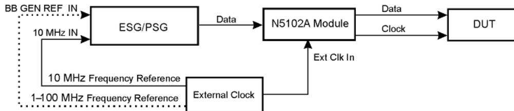
**NOTE:** Use only one of the two signal generator frequency reference inputs.
