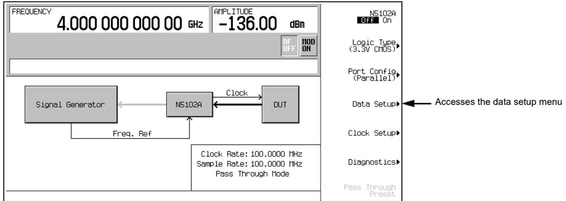
This softkey menu accesses the various parameters that govern the data received by the PSG. The status area of the display shows the number of data lines used for both I and Q along with the clock position relative to the data. **Figure 12-20** shows the data setup menu structure.
