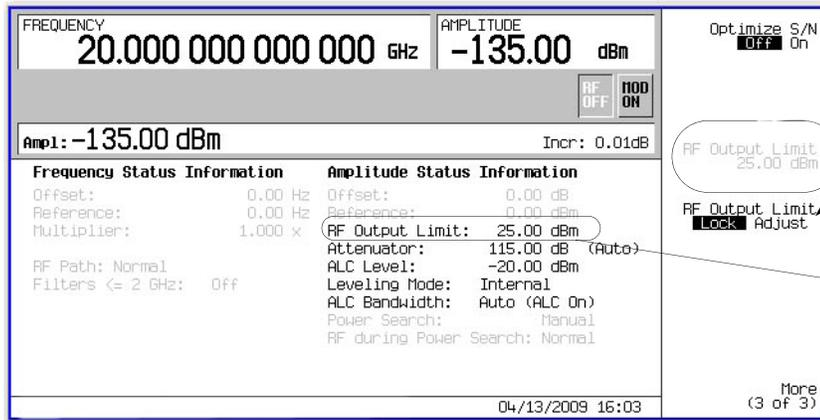
This softkey is only active when the RF Output Limit softkey is set to "Adjust".
