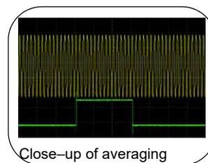
The ALC samples the waveform when the marker signal goes high, and uses the average of the sampled waveform to set the ALC circuitry.
