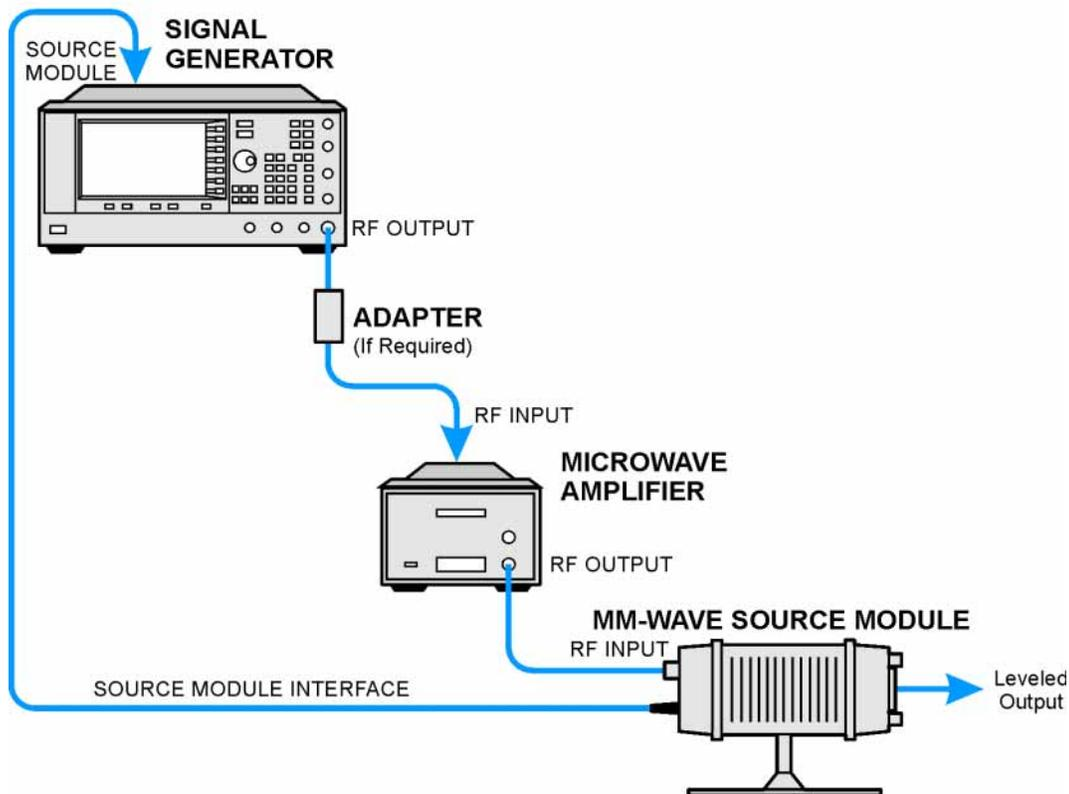
**Figure 12-22** Setup for E8267D PSG and E8257D PSG with Option 1EA, 1EU, or 521
