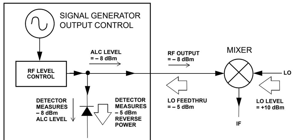
The internally leveled signal generator RF output (and ALC level) is  $-8$  dBm. The mixer is driven with an LO of  $+10$  dBm and has an LO-to-RF isolation of  $15$  dB. The resulting LO feedthrough of  $-5$  dBm enters the signal generator's RF output connector and arrives at the internal detector.
