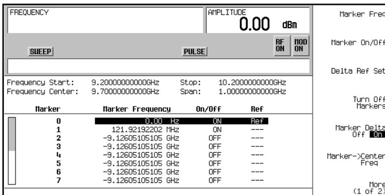
5. Move the cursor back to marker 1 and press **Marker Freq**. Turn the front panel knob while observing marker 1 on the 8757D.
