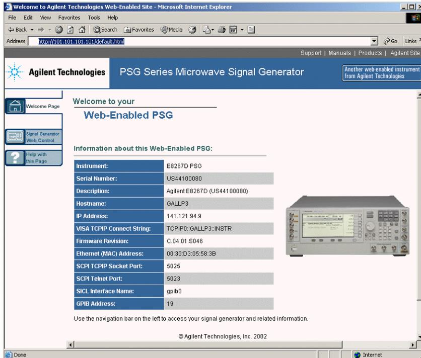
7. Click the Signal Generator Web Control menu button on the left of the page. A new web page will be displayed as shown below in **Figure 2-14**.
