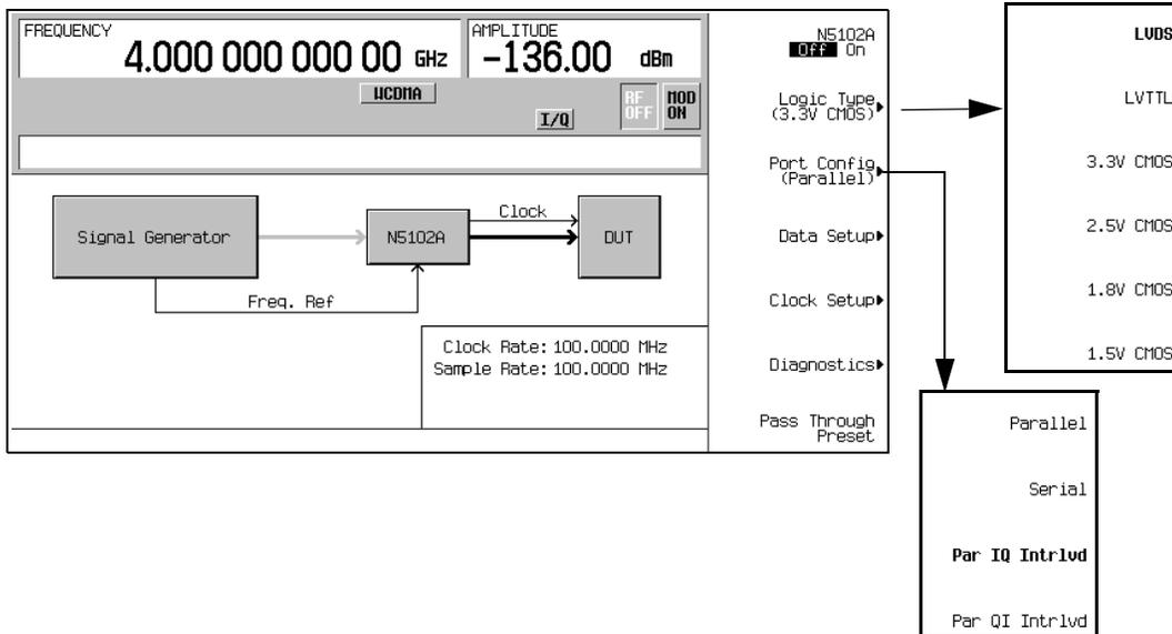
1. Refer to **Figure 12-10**. Press the **Logic Type** softkey.
