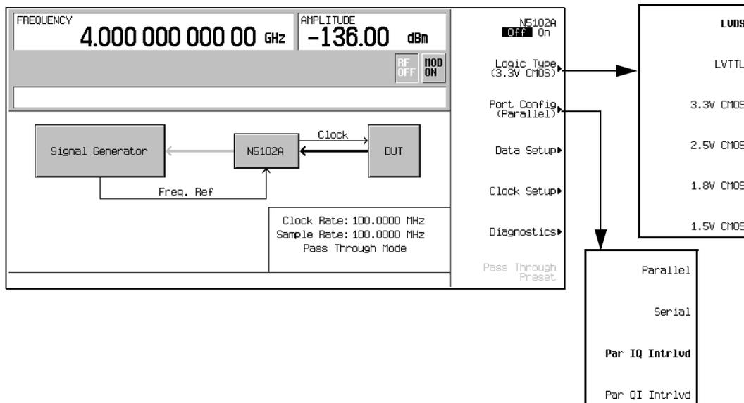
1. Refer to **Figure 12-16**. Press the **Logic Type** softkey.
