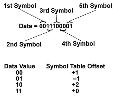
When applied to the user-defined default 4QAM I/Q map, starting from the 1st symbol (data 00), the differential encoding transitions for the data stream (in 2-bit symbols) 0011100001 appear in the previous illustration.
