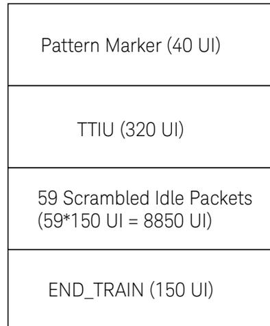
Figure 7 Structure of Train\_Tx pattern sent during Train\_Tx-SNW
