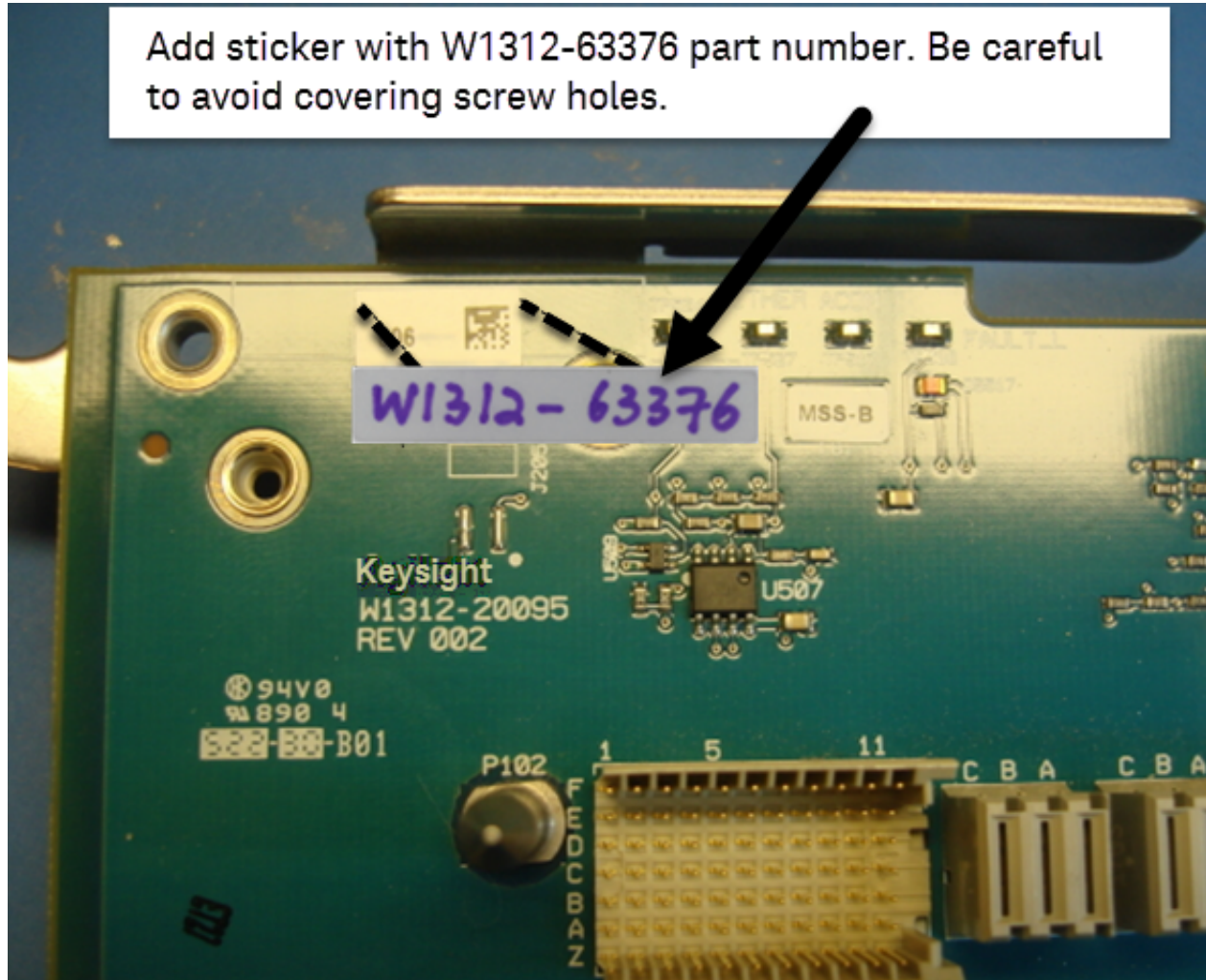
Figure A-6 Adding sticker to new board number W1312-63376—Top Side View
