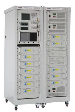
The Rflight NTPIM-XXXX Series PIM test system utilizes Keysight power meters and spectrum analyzers In order to test for the intermodulation of passive devices. The maximum output power of the test port is over +48dBm, with +53dBm available as an option, maximum intermodulation distortion accuracy is -168dBc.
