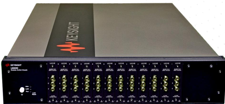
The Keysight L8990M Modular Signal Routing Solution provides a simple and flexible platform for RF switching and signal conditioning with signal frequencies up to 67 GHz. The L8990M platform can support up to 128 switch channels in a 2U rack-mountable enclosure, and 196 switch channels in a 4U high enclosure. This flexibility provides the capability to route and condition signals to test a wide range of RF and telecommunication products and devices.
