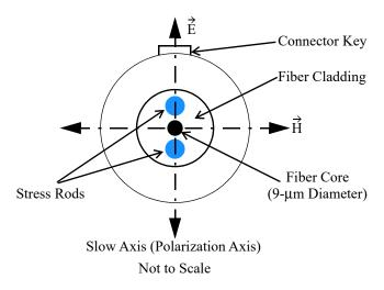
Figure 5 PMF Output Connector
