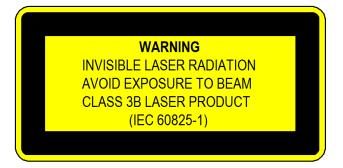
Figure 1 Class 3B Safety Label - Keysight 81602A
