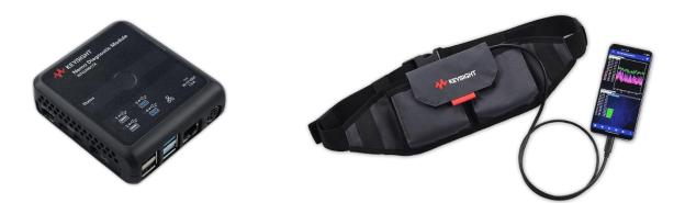
Nemo Diagnostic Module can be carried in a compact hip belt with a wired connection to the phone.
