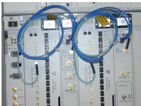
Figure 49 Clock Distribution of two 7G/13.5G Systems in one Mainframe
