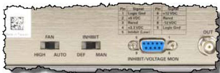
**Figure 56** Rear Panel Inhibit Switch and DB-9 Connector
