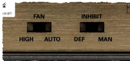
Chassis Rear Panel Fan and Inhibit Switches
