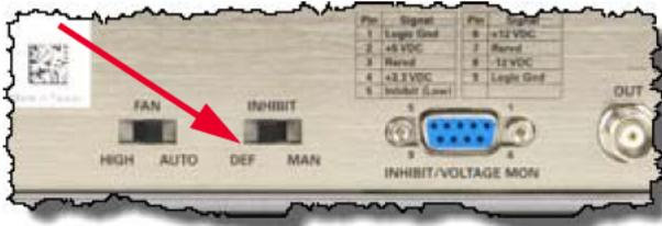
Chassis Rear Panel Fan and Inhibit Switches
