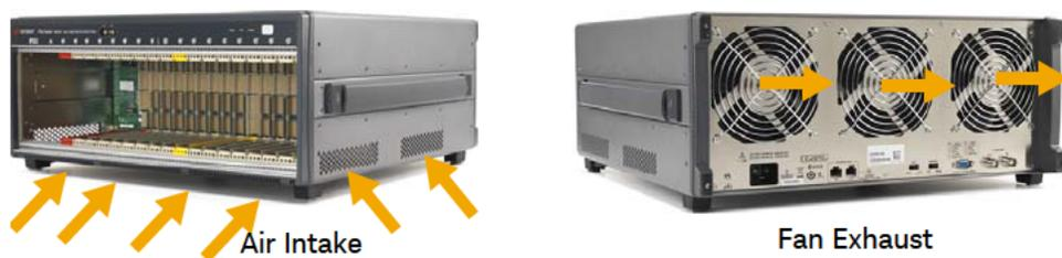
**Figure 21** M9018B and M9019A Chassis Air Flow
