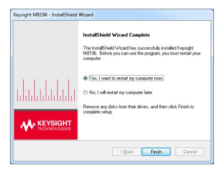
14. Click **Finish** to restart your system. Do not connect the AXIe chassis to your system using the PCIe or USB cable during this reboot.
